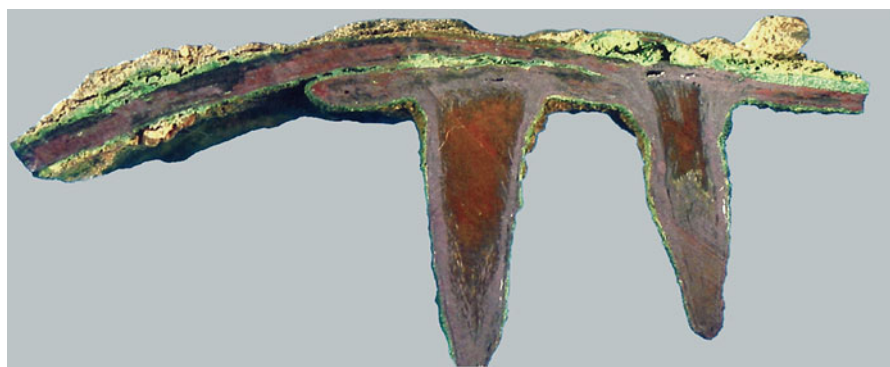
Fig. 14.16 Detail of sample taken from the Pepi I statue demonstrating the way the metal sheets were riveted together
