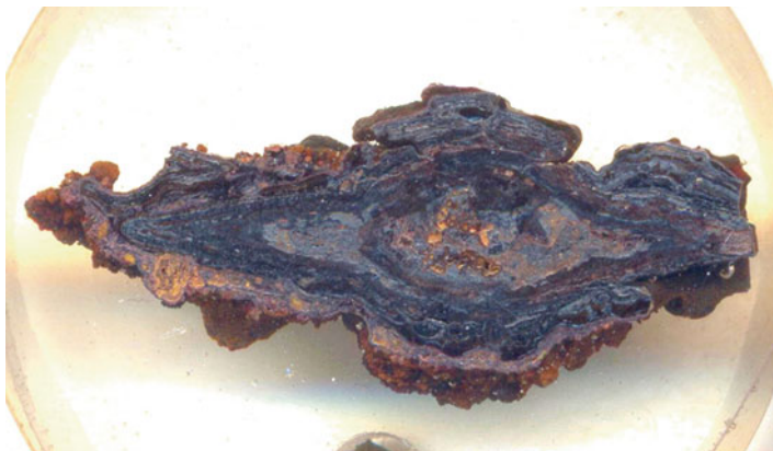
Fig. 14.2 Cross section of the iron blade. Evidence of the limits of the original surface are still preserved within corrosion layers
