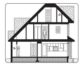
In a multilevel home or business, when a floor covering in one of the upper rooms is impacted, by dropping an object or moving furniture, for example, the impact creates a vibration that travels through the floor, subfloor, and through the ceiling to the room below. These vibrations result in unwanted and annoying sounds in those
