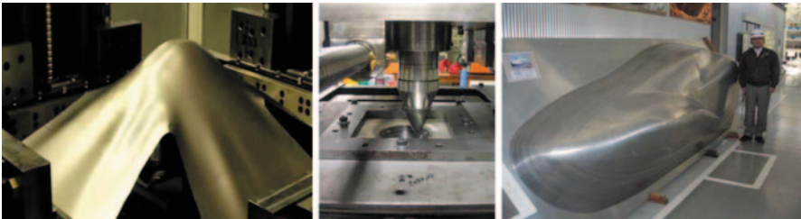
Fig. 7 An example application of ISF: a 1/8 scale model of the front section of a Shinkansen ( Bullet Train ) made by Amino in Japan
