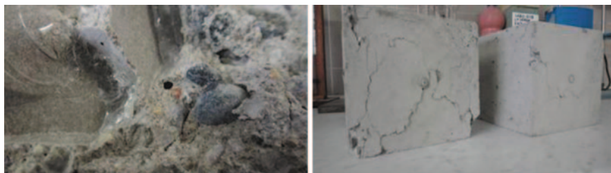
Fig. 1 Left test rupture in detail. Right test: flat glass breaking 30% at 28 days
