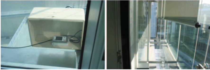
Fig. 2 Probe on the interior windows ( left ) and the air gap ( right )
