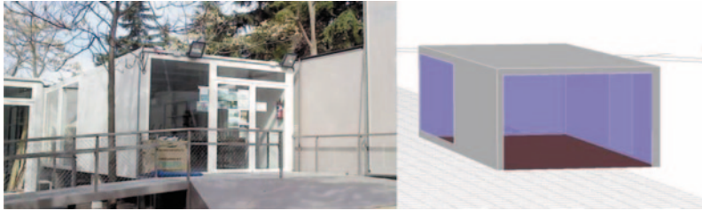
Fig. 10 Comparison between studied real test cell and Ecotect software simulation image
