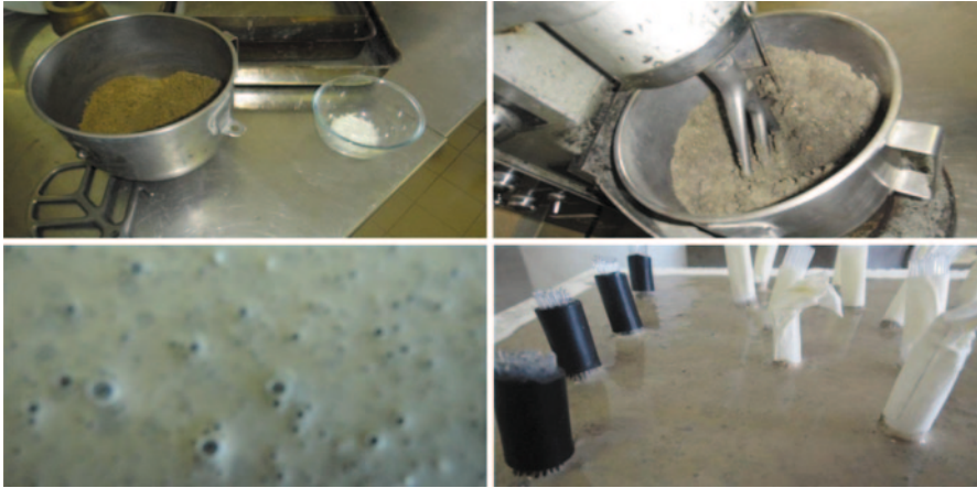
Fig. 2 Optical fiber/concrete manufacturing process
