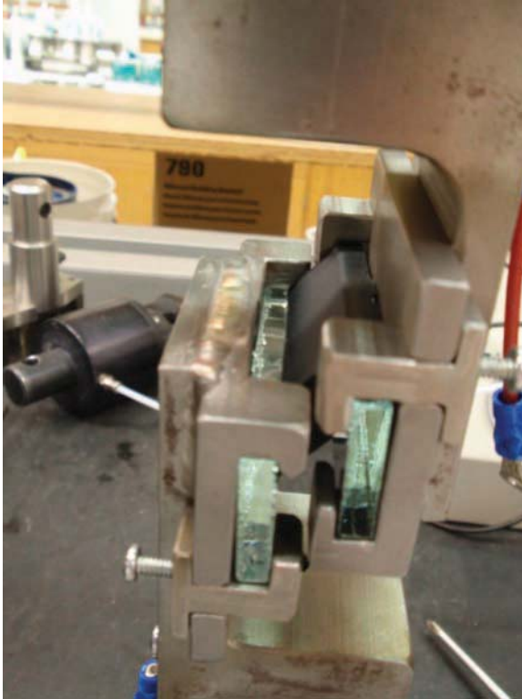
FIG. 10—Typical shear adhesion sample set up as installed on a tensile testing machine.
