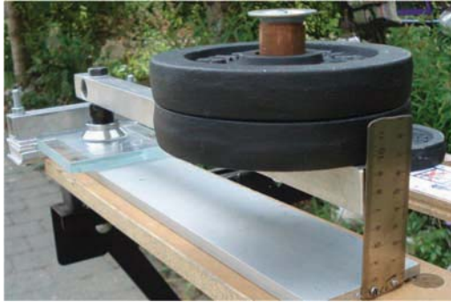
FIG. 13—Cantilever pull-off test equipment used in outdoor exposure in southern Germany.
