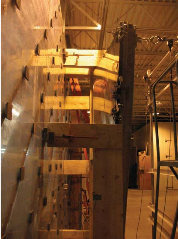
FIG. 5— 120 \times 60 \times 1 in 3 . ( 1.5 \times 3.0 m 2 \times 25 mm). Full-scale test assembly 2 in partial test frame.
