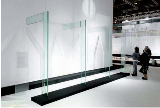
FIG. 5—Design studies at glasstec 2010 in Düsseldorf, Germany: transparent bonded glass frame corners.
