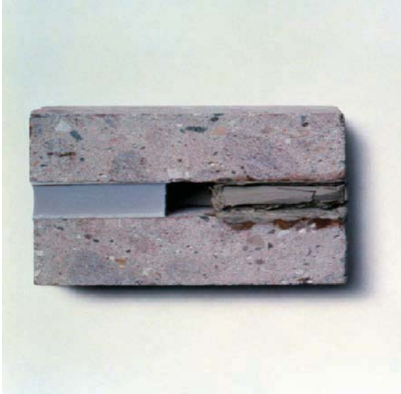
FIG. 3—Silicone versus organic sealant after 5000 h QUV exposure.
