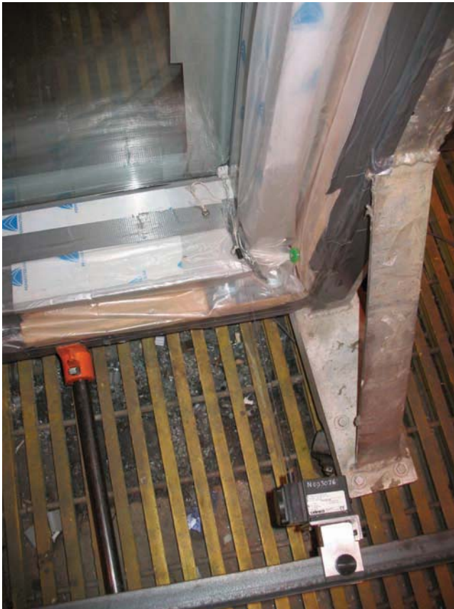
FIG. 14—One of four LVDTs measuring bending in the full-scale test specimen.
