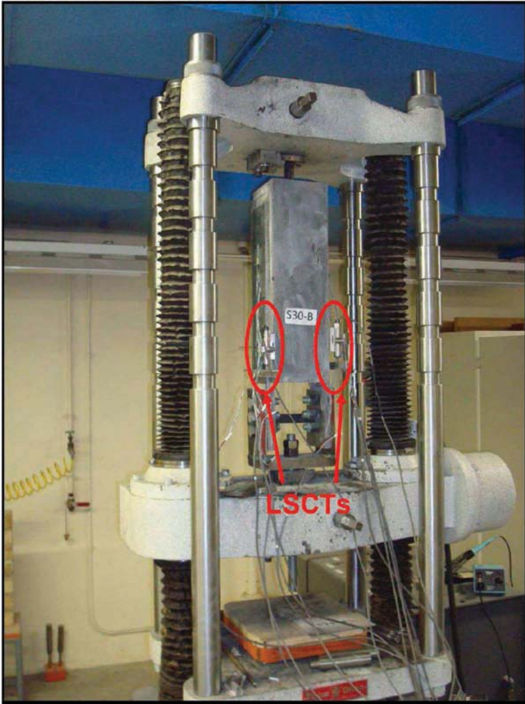
FIG. 4—Double-lap shear specimen testing load setup.
