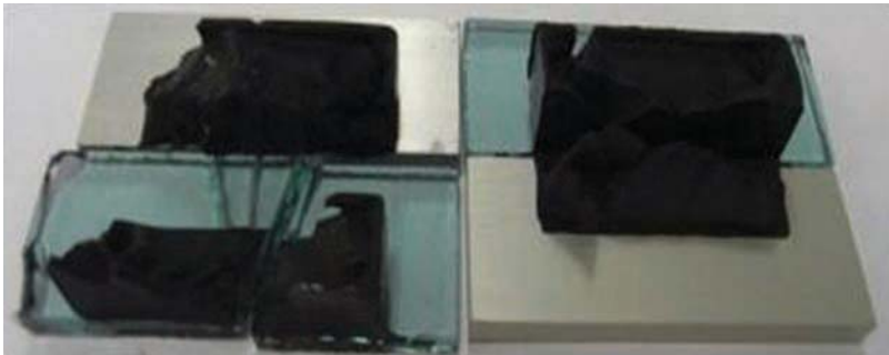
FIG. 3—Initial cohesive failure mode of locally compounded one-part structural silicone.
