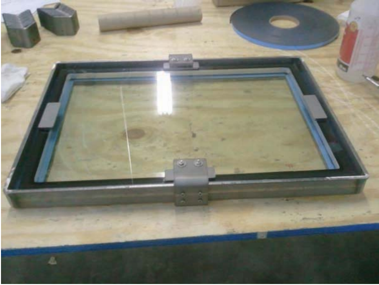
FIG. 9— 14 \times 20 \text{ in.}^2 ( 350 \times 500 \text{ mm}^2 ) small test frame with IGU installed.
