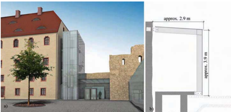
FIG. 3—New glass structures for the historic courtyard: (a) visualization (Bauconcept Planungsgesellschaft mbH), and (b) Vertical section through new glass corridor (GSK – Glas Statik Konstruktion GmbH).
