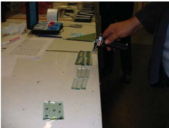
FIG. 4—Application of Pyrosil ® .
