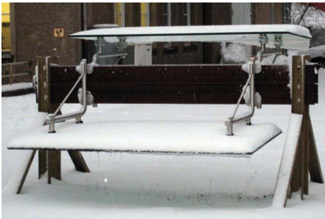
FIG. 10—Outdoor overhead glazing test: in the foreground the suspended pane, in the background the supported pane.
