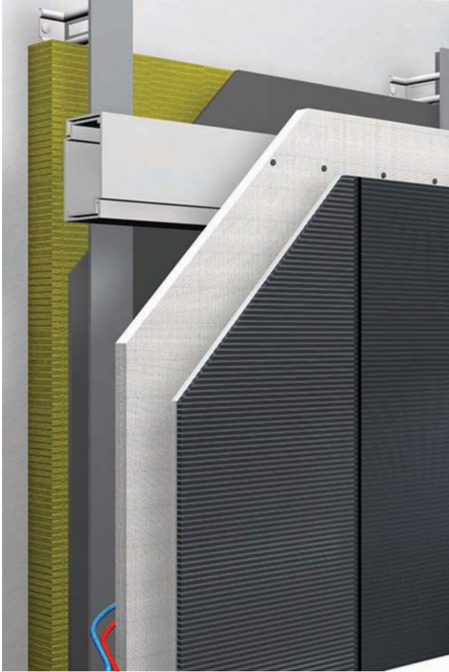
FIG. 19—Construction of a facade for generating electricity.
