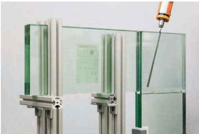
FIG. 14—Applying a transparent adhesive to a sample component with the help of a special injector.
