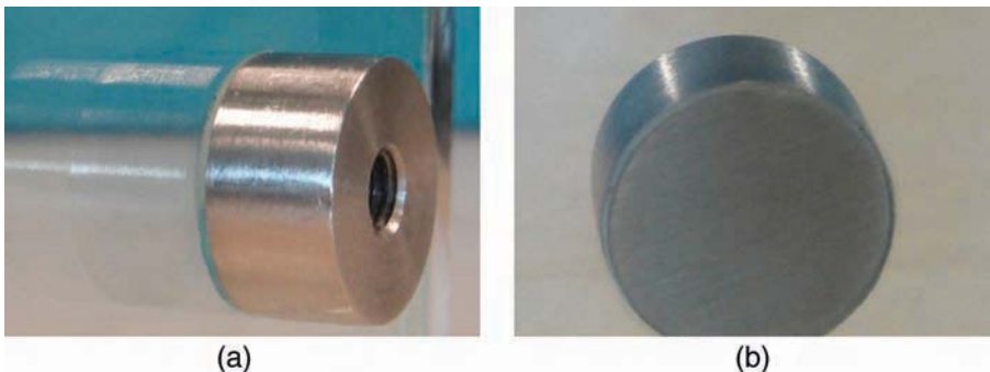
FIG. 3—Stainless steel button attached to glass with TSSA (seen from side and rear face).
