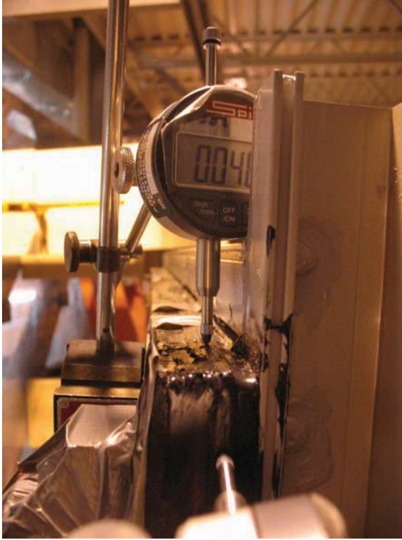
FIG. 6—Dial gauge used to measure relative displacement between glass panes in full-scale test assembly 2.
