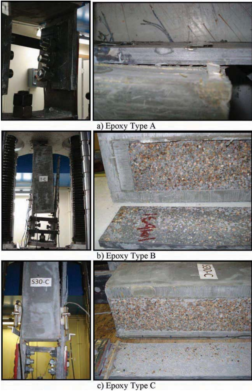
FIG. 7—Photographs at failure for double shear test specimens.
