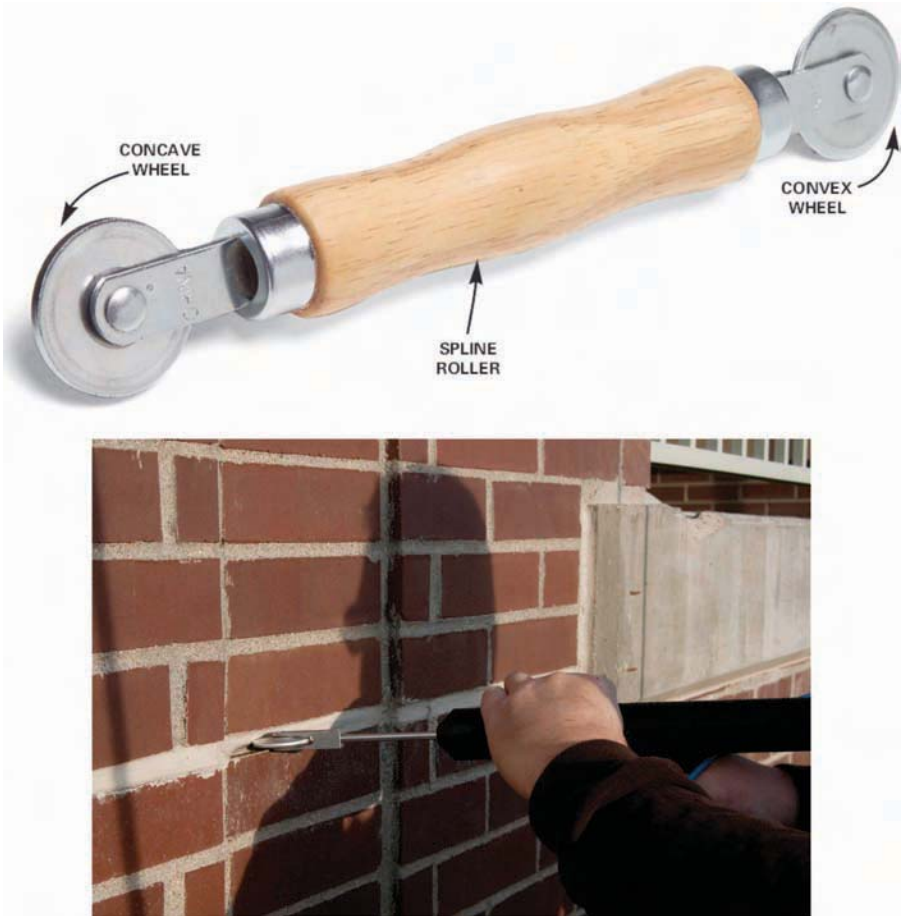
FIG. 1—Upper portion depicts an uncontrolled “screen roller” type device used in procedural section 7.3, lower portion is the controlled force device per section 7.4.
