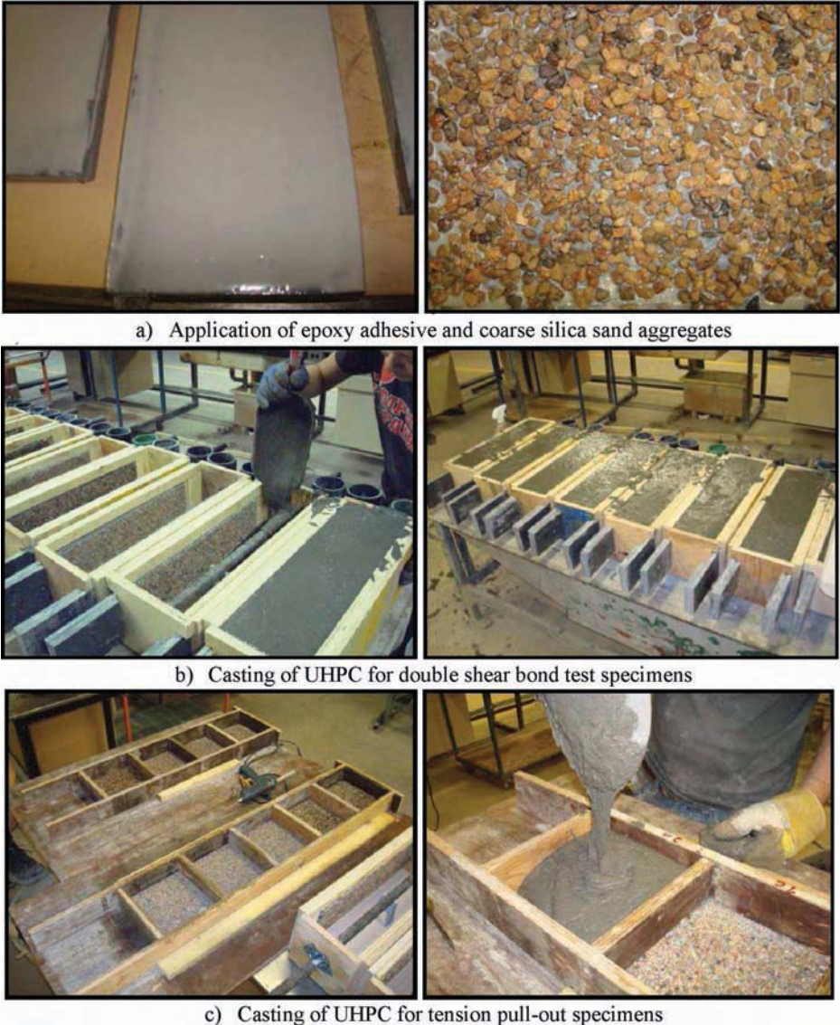
FIG. 1—Fabrication of test specimens.
