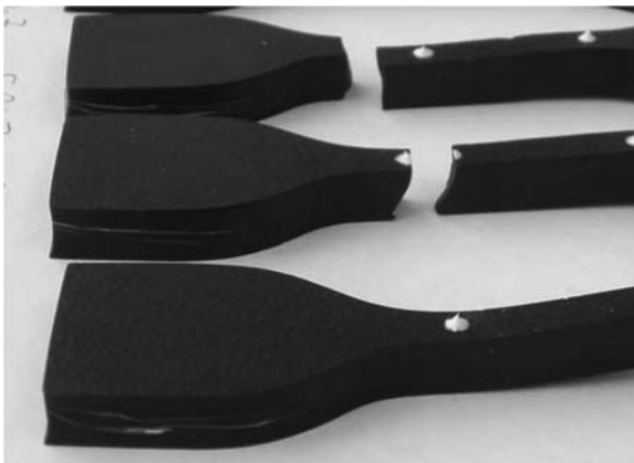
FIG. 7—Specimens featuring incomplete mixing.
