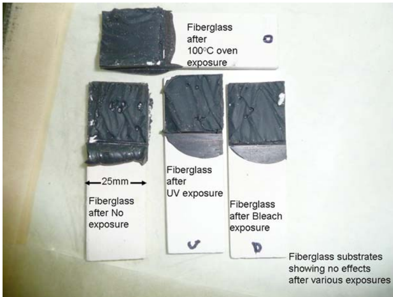
FIG. 13—Fiberglass specimens after UV, oven, and bleach exposures and control.
