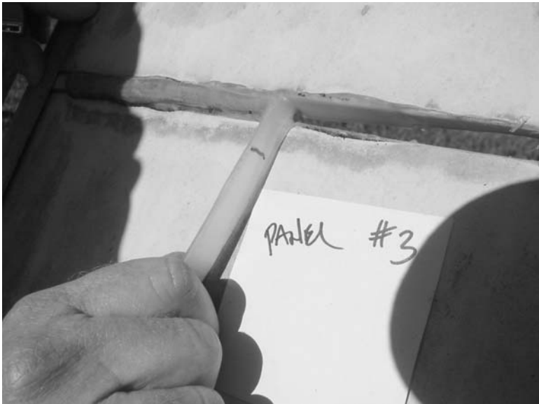
FIG. 5—Adhesion check by hand Pull, during.
