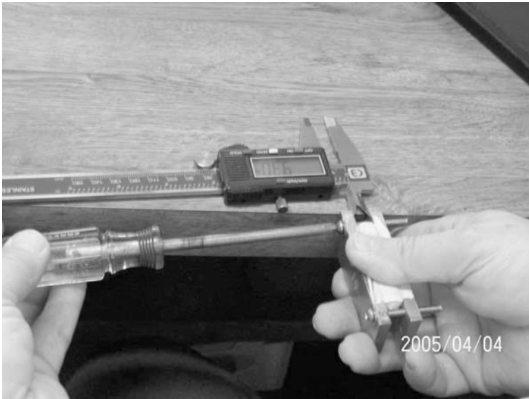
FIG. 3—Setting compression with screw.
