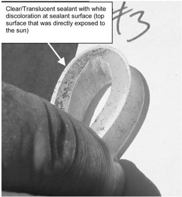
FIG. 35—Silicone sealant #3, surface discoloration.
