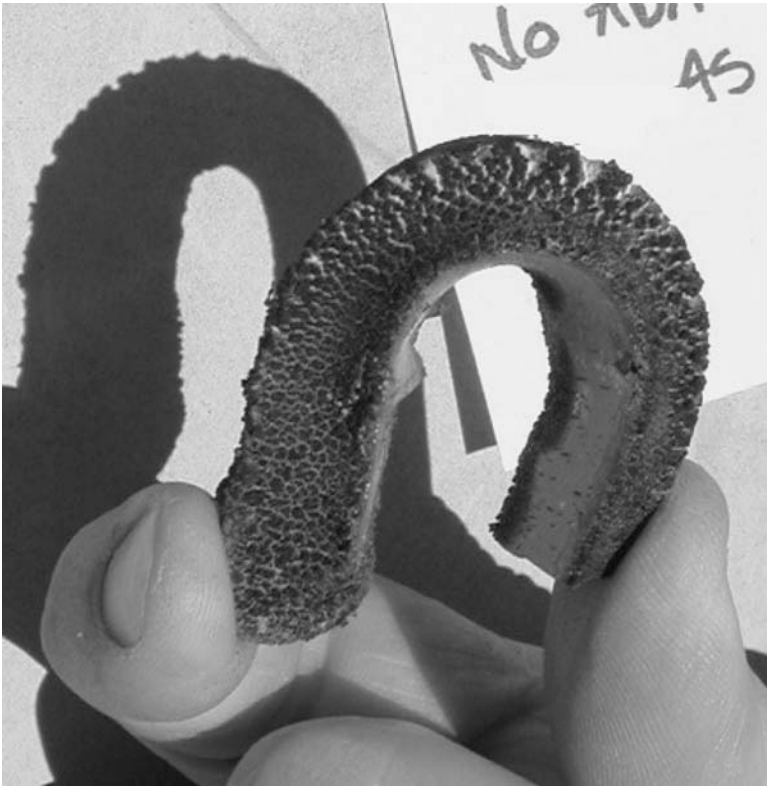
FIG. 7—180° manual bend of sealant (rated Good).
