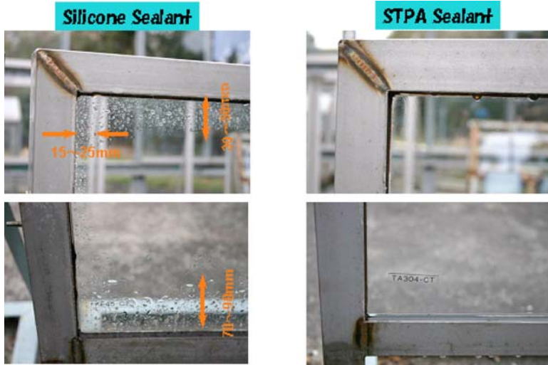
FIG. 14—Contamination test results on window shaped specimens (outdoor exposure for 812 days; photos taken after spraying the surface with water).
