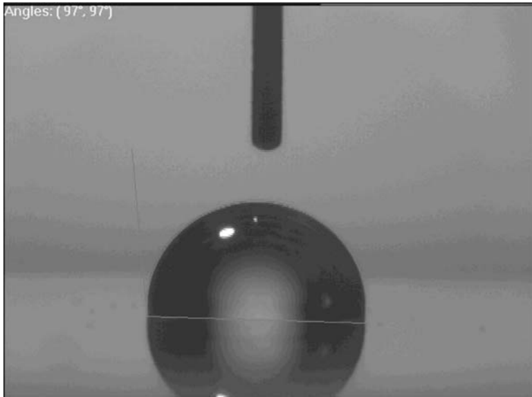
FIG. 1—The tangent angle of a bead of water on an oily surface at the point of contact of the water and the oily surface is typically between 90^\circ and 110^\circ . This angle is called the contact angle.
