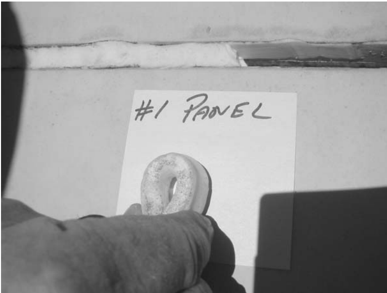
FIG. 6—180° manual bend of sealant (rated Excellent ).
