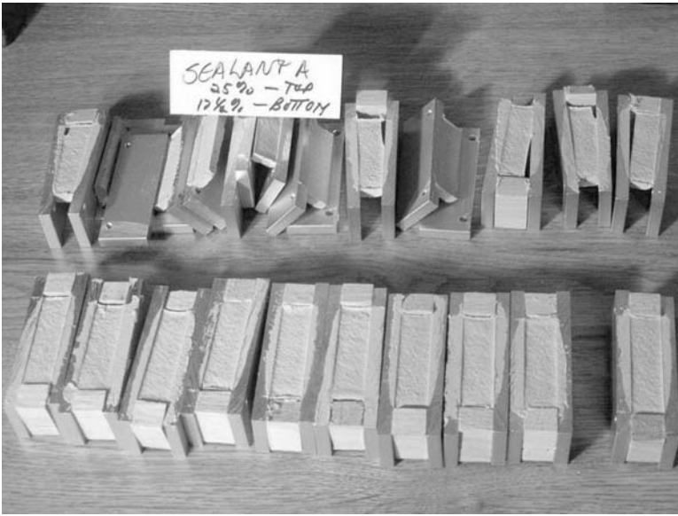
FIG. 7—Failures after the first extension at half the rated movement.
