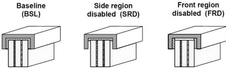
FIG. 11—U-type bonding test configurations.
