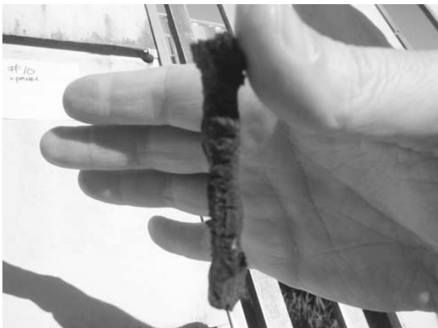
FIG. 42—Polyurethane sealant #10, reversion.
