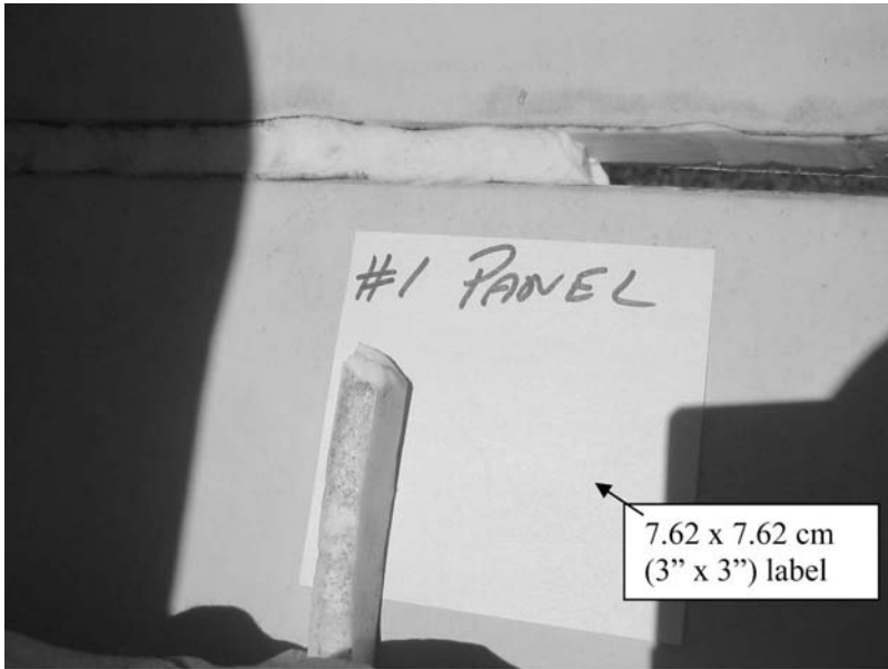
FIG. 10—Sealant immediately after release of 180° manual bend.
