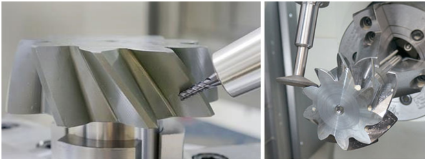
Fig. 10 Rough-cutting and finish-grinding of IPB pinion teeth
