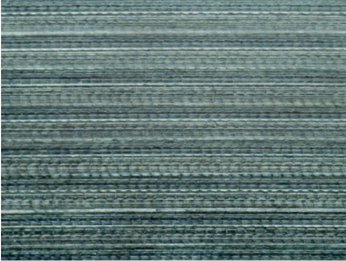
Fig. 16 Typical plane tooth flank of an IPB wheel finished by one path of cutting with a \varnothing 8 mm flat end mill
