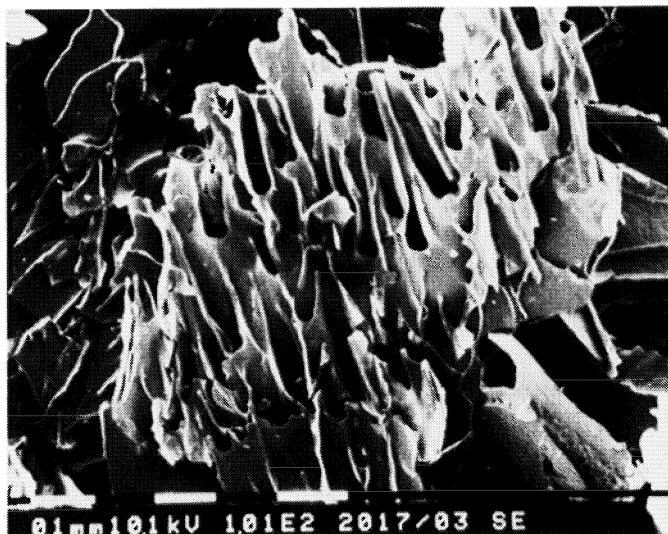
Figure 13. SEM photograph of corticosteroid after freeze-drying. The freezing temperature was -60^{\circ}\text{C} .
