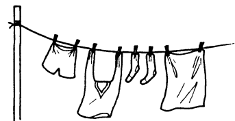
Figure 6.1g A washing line is a common tensile structure
