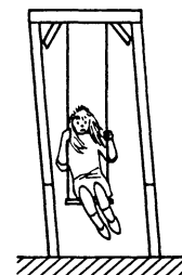
Figure 1.9c Bracing connections fail
