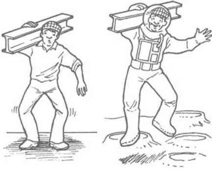
Figure 2.1 Because of gravity, objects with the same mass only exert a sixth of the force on the moon
