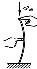
Figure 8.4b A horizontal load is applied
