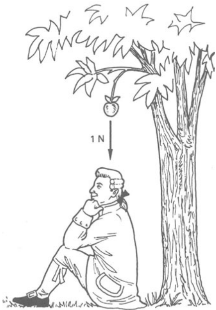
Figure 2.2 A newton is roughly the force exerted on earth by a (stationary) apple
