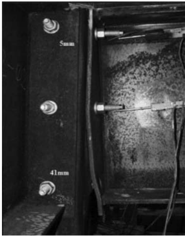
Figure 11. End plate bending.
