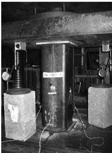
Figure 7. Test setup of CFCFST column specimen.
