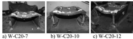
Figure 13. Deformed shape of the prototypes after compressive tests at ambient temperature.
