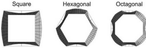
Figure 4. Critical local buckling mode shapes of even-sided polygonal columns.
