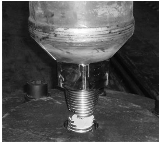
Figure 8. Bolt M80-A Nuclos after being tested.
