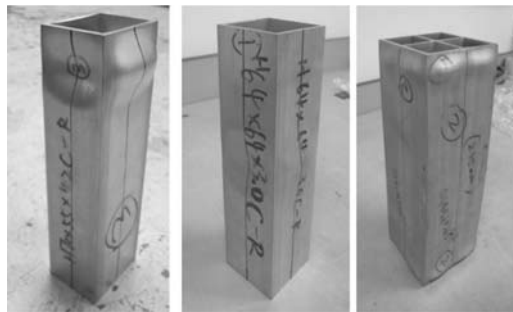
Figure 9. Stub column failure modes of specimens H70 × 55 × 4.2C-R, H64 × 64 × 3.0C-R and +H95 × 95 × 4.3C.
