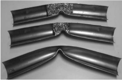
Figure 7. The interior of tubes after tests. From front to back: a hollow tube (specimen 9), hybrid tubes with 50 mm and 75 mm long foam inserts (specimens 11 and 13).
