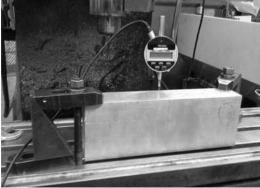
Figure 3. Measurement of initial local geometric imperfections.
