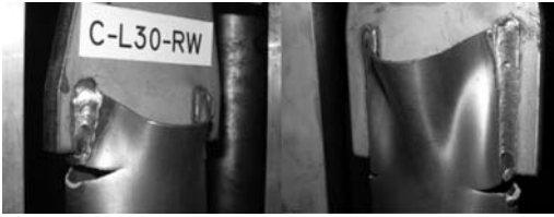
Figure 8. Shear lag failure observed in specimens with different weld lengths.
