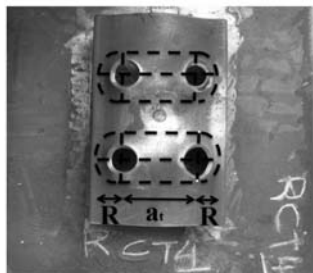
(b) Failure mode A
