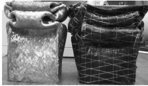
Figure 7. Typical failure mode of SHS and CFRP-SHS subject to large deformation axial loading (Bambach and Elchalakani 2007).
