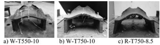
Figure 18. Deformed shape of the prototypes after tensile tests at elevated temperatures.
