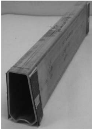
Figure 6. Failure mode of CFRP strengthened ferritic stainless steel F120 × 40 × 3-EOF-f1 section subjected to EOF loading condition.
