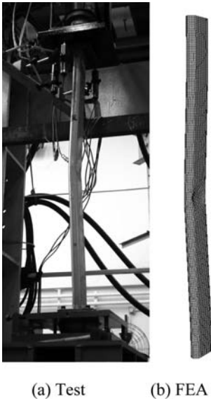
Figure 4. Comparison of experimental and FEA deformed shapes for specimen B1200.
