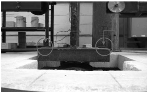
Figure 4. Wires used to measure the displacement for elevated temperature tests.
