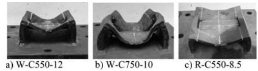
Figure 19. Deformed shape of the prototypes after compressive tests at elevated temperatures.
