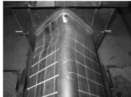
(b) Local buckling (cold-formed No.4).
