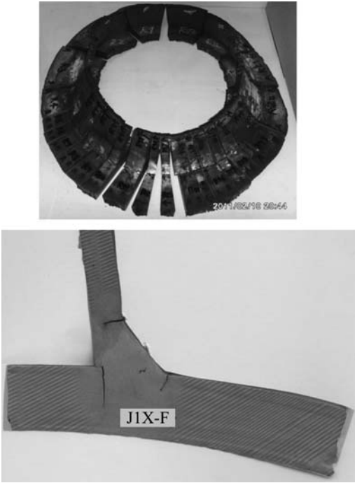
Figure 9. (a) Post-test sectioning of the brace-to-chord intersection region; and (b) root cracking in the specimen J1X-F.
