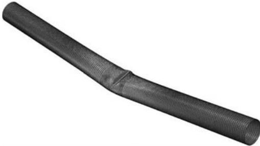
Figure 13. Buckled shape of 5m-long tube of section AA under axial compression.
