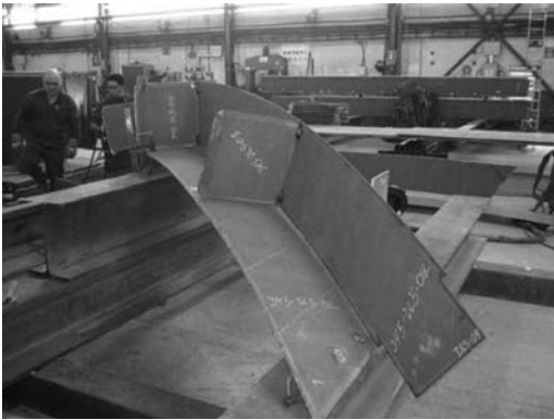
Figure 14. Assembly and welding of a diagonal
