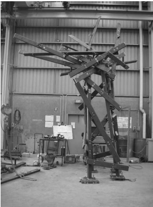
Figure 14. Trial assembly in the fabricator's works.
