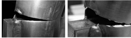
Figure 6. Failure types for Return Weld (RW) and No-return Weld (NW) cases.
