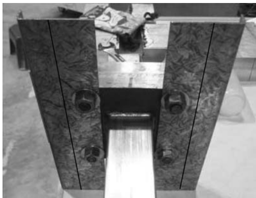
Figure 4. Two steel stripes bolted to the upper end plate with two parallel lines drawn.
