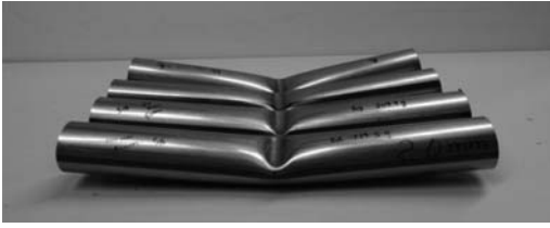
Figure 6. The deformation of tubes when the carriage dropped from 2.0 m. From the front to back: specimens 15, 13, 11 and 9 with foam insert length of 100 mm, 75 mm, 75 mm and 0 mm respectively.
