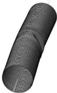
Figure 8. Buckled shape for the B4 specimen in comparison with the FE model.
