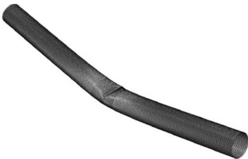
Figure 16. Buckled shape of 5m-long tube with section AB under combined compression and bending.
