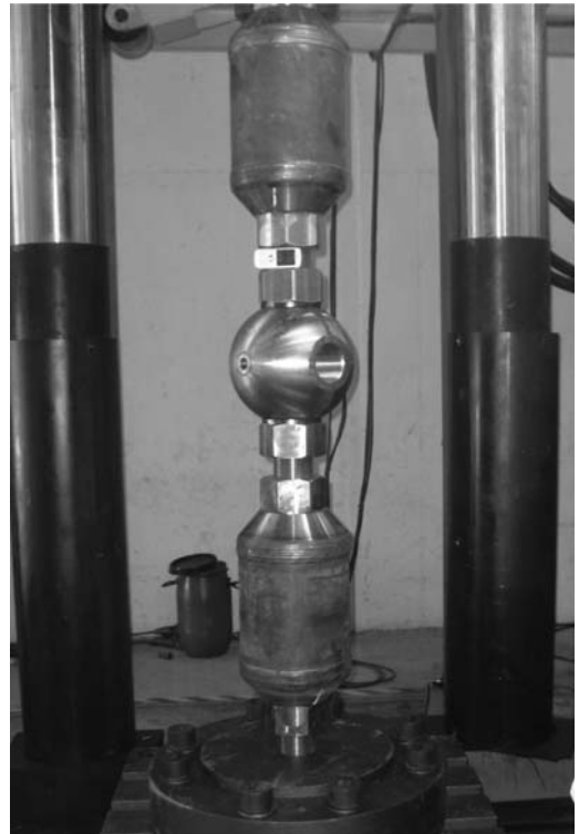
Figure 6. Experimental set-up for the M80-A Nuclos joint.
