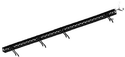
Figure 6. Vibration mode associated with the 1st footbridge natural frequency ( f_{01} = 1.61 Hz).
