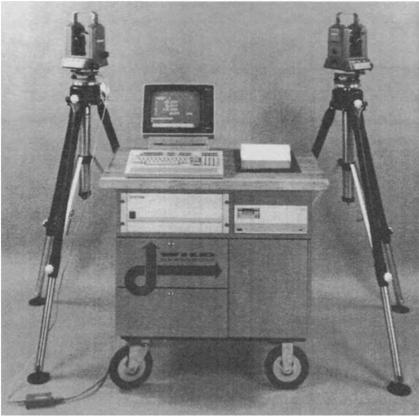
Figure 31-18. Coordinate-analyzing theodolite system. (Courtesy of Wild Heerbrugg Instruments, Inc.)
