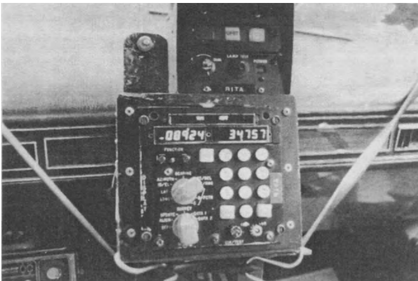
Figure 14-8. Control and display unit for Litton Auto-Surveyor.
