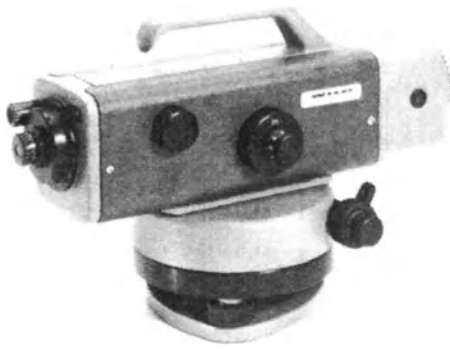
Figure 31-10. Wild N-3 tilting level. (Courtesy of Wild Heerbrugg Instrument, Inc.)
