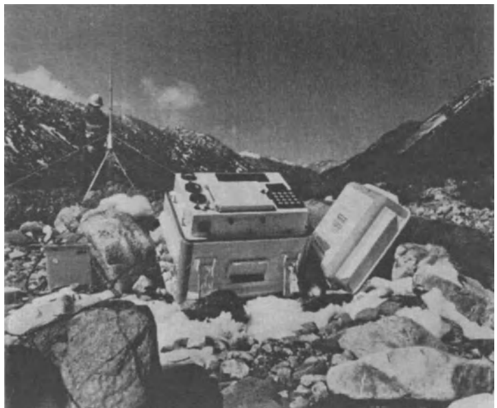
Figure 14-22. Magnavox MX 1502 geociever satellite surveyor field site setup. (Courtesy of Magnavox Advanced Products and Systems Co.)
