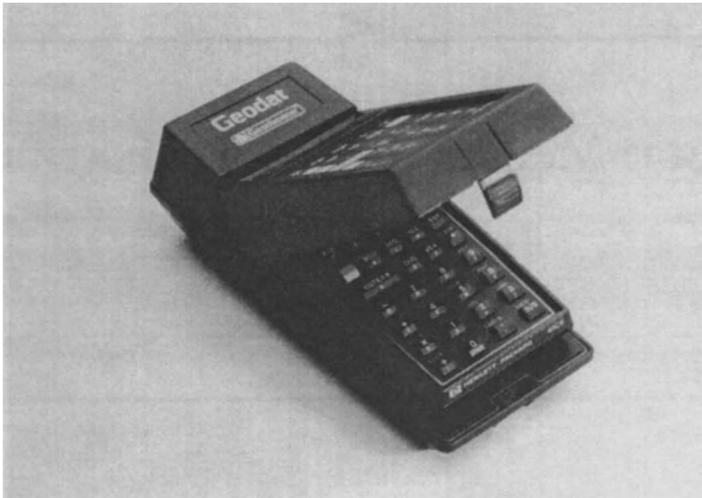
Figure 5-14. Data collector or electronic field book. Geodat 126 uses HP-41CX calculator as “administrative system” (display, keyboard, calculating capacity, and memory module) and adds HP Interface Loop, RS-232C interface, and additional memory for storing measurement data, file handling, and special programs. (Courtesy of Geodimeter.)
