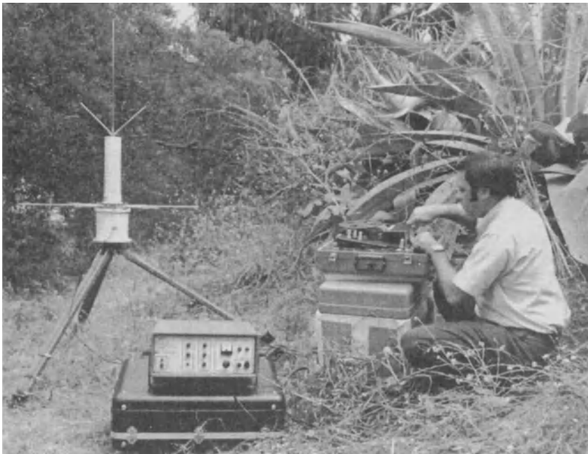
Figure 14-17. Magnavox ANPRR-14 geociever. (Courtesy of Magnavox Advanced Products and Systems Co.)
