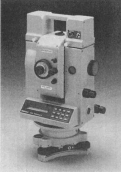
Figure 5-13. Manual total station, combining an EDM instrument, theodolite, and preprogrammed calculator in a single instrument. After zenith angle is keyed in, display shows slope distance, horizontal distance, and vertical distance in turn. Instrument offers tracking mode, stake-out mode, and distance-averaging mode. Optional cordless control unit is available. (Courtesy of Pentax Corp.)
