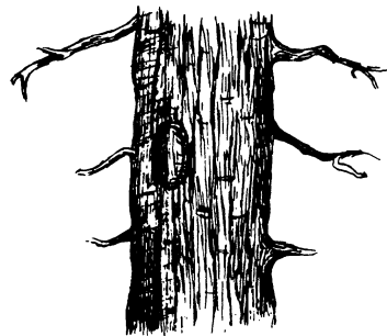
Figure 30-13. Line tree with blaze. ( Manual of Instructions for the Survey of the Public Lands of the United States—1973 . 1975. Reprint. Rancho Cordova, CA: Landmark Enterprises.)
