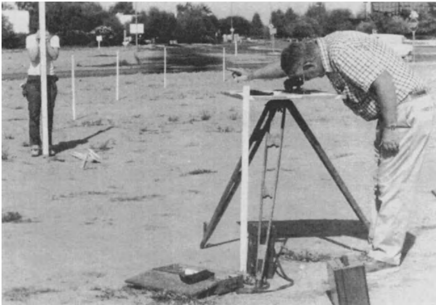
Figure 22-8. Using the planetable in layout mode to stake a curved entrance drive.
