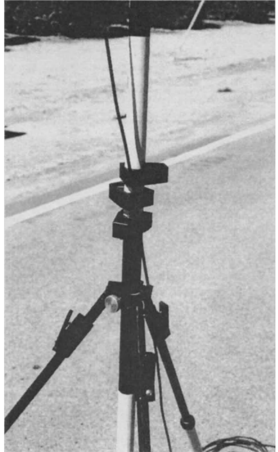
Figure 15-23. GPS rod with three bubbles.
