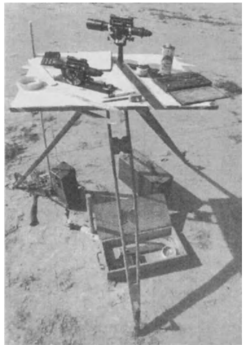
Figure 22-1. Planetable with two old-style alidades and some ancillary equipment.
