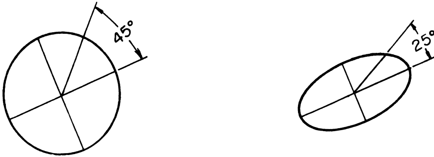
Figure 18-13. When a circle is projected as a noncircular ellipse, the angle between two radial lines will be deformed, except for the two perpendicular that become the ellipse axes.
