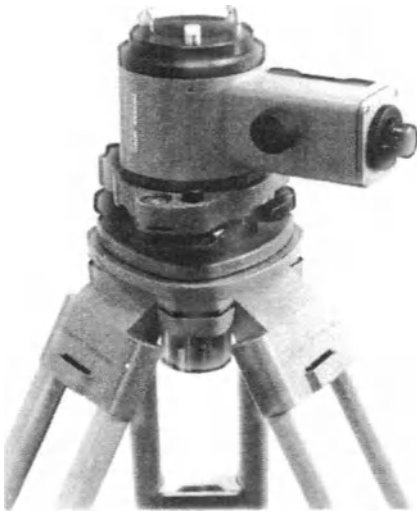
Figure 29-3. ZNL automatic nadir plummet. (Courtesy of Wild Heerbrug Instruments, Inc.)
