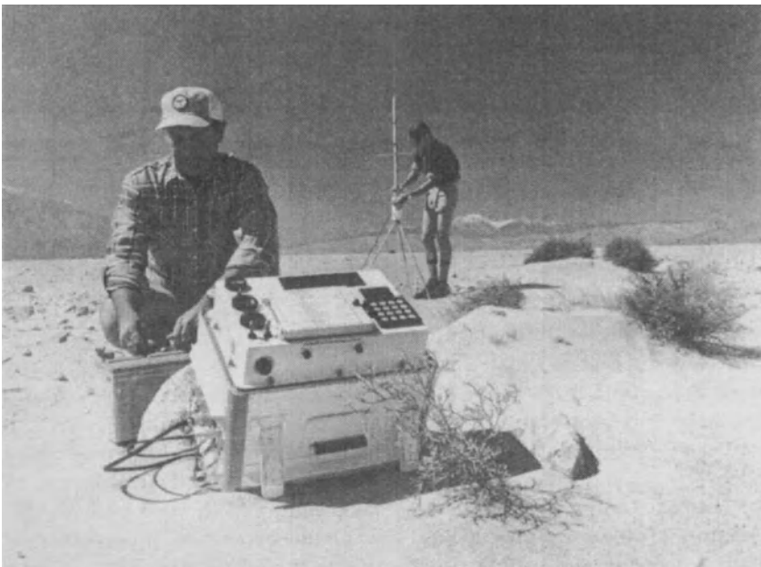
Figure 13-23. Magnavox MX 1502 georeceiver/satellite surveyor. Portable, battery-operated precise point-positioning and translocation system (Courtesy of Magnavox Advanced Products and Systems Co.)
