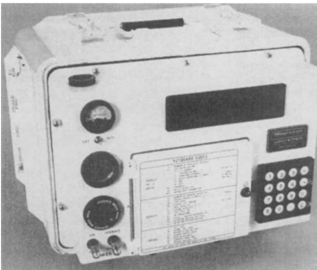
Figure 14-24. Receiver control panel for Magnavox MX 1502 georeceiver satellite surveyor. (Courtesy of Magnavox Advanced Products and Systems Co.)
