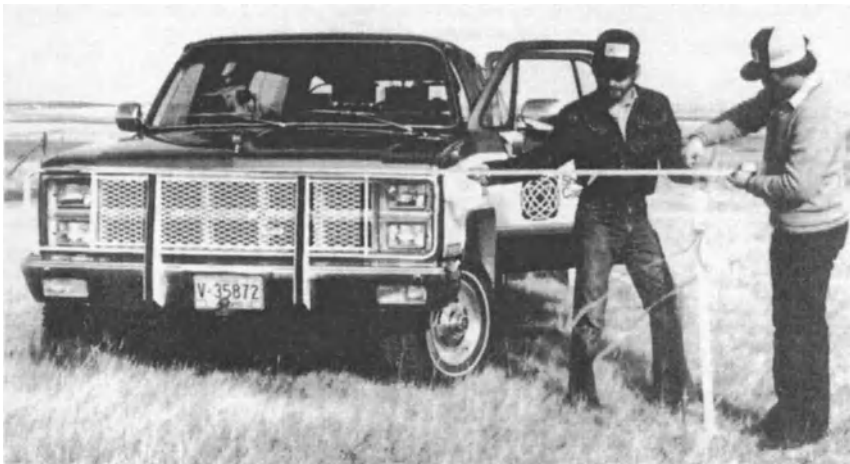
Figure 14-13. Measuring offset from vehicle measuring mark to survey point. (Courtesy of Shell Canada Resources, Ltd.)
