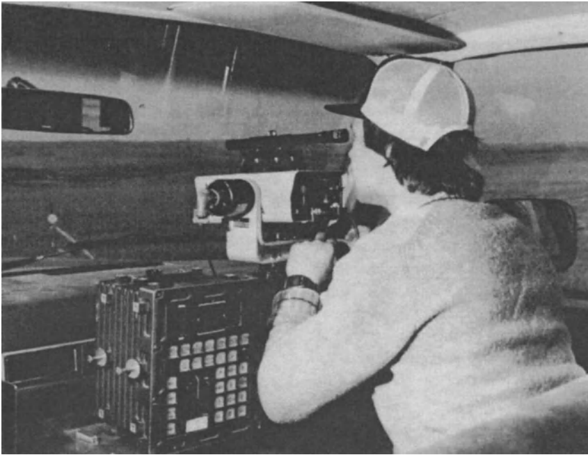
Figure 14-14. Offset measurement to survey point using electronic distance-measuring instrument. (Courtesy of Shell Canada Resources, Ltd.)
