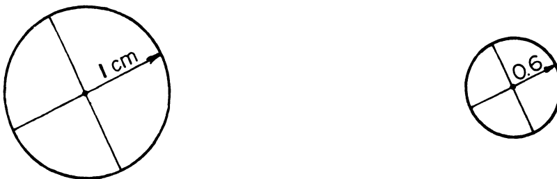
Figure 18-11. In conformal projections, a circle on a globe, at left, will project as another circle (a special kind of ellipse). A scale factor of 0.6 is illustrated.
