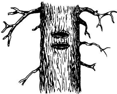
Figure 30-12. Line tree with hack marks. ( Manual of Instructions for the Survey of the Public Lands of the United States—1973 . 1975. Reprint. Rancho Cordova, CA: Landmark Enterprises.)
