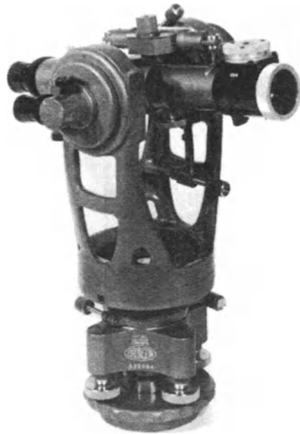
Figure 31-17. Brunson 76R telescope transit square. (Courtesy of Brunson Instrument Co.)
