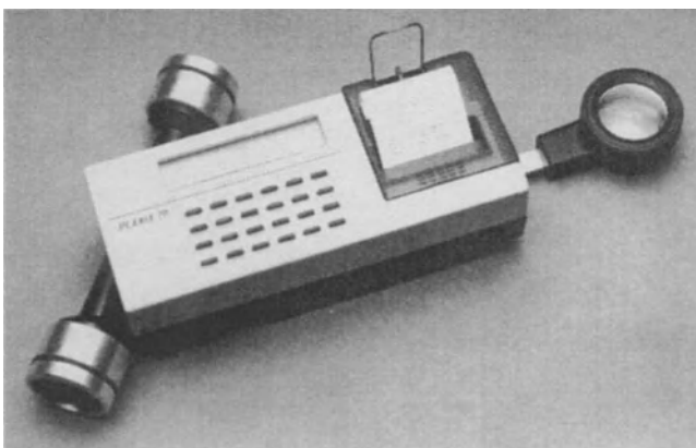
Figure 9-10. Planix electronic planimeter. (Courtesy of the Lietz Co.)
