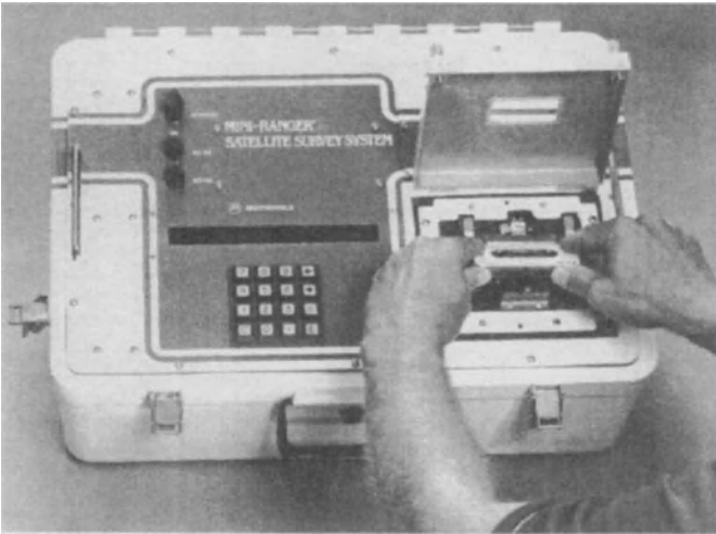
Figure 14-23. Data tape cassette for Motorola Mini-Ranger satellite survey system. (Courtesy of Motorola, Government Electronics Group.)
