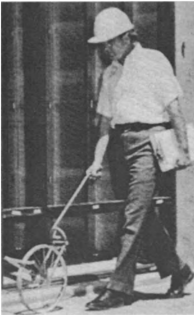
Figure 4-1. Measuring wheel. (Courtesy of Rolatape Corporation.)
