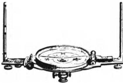
Figure 30-4. Surveyor's compass. (Courtesy of F. D. Uzes.)
