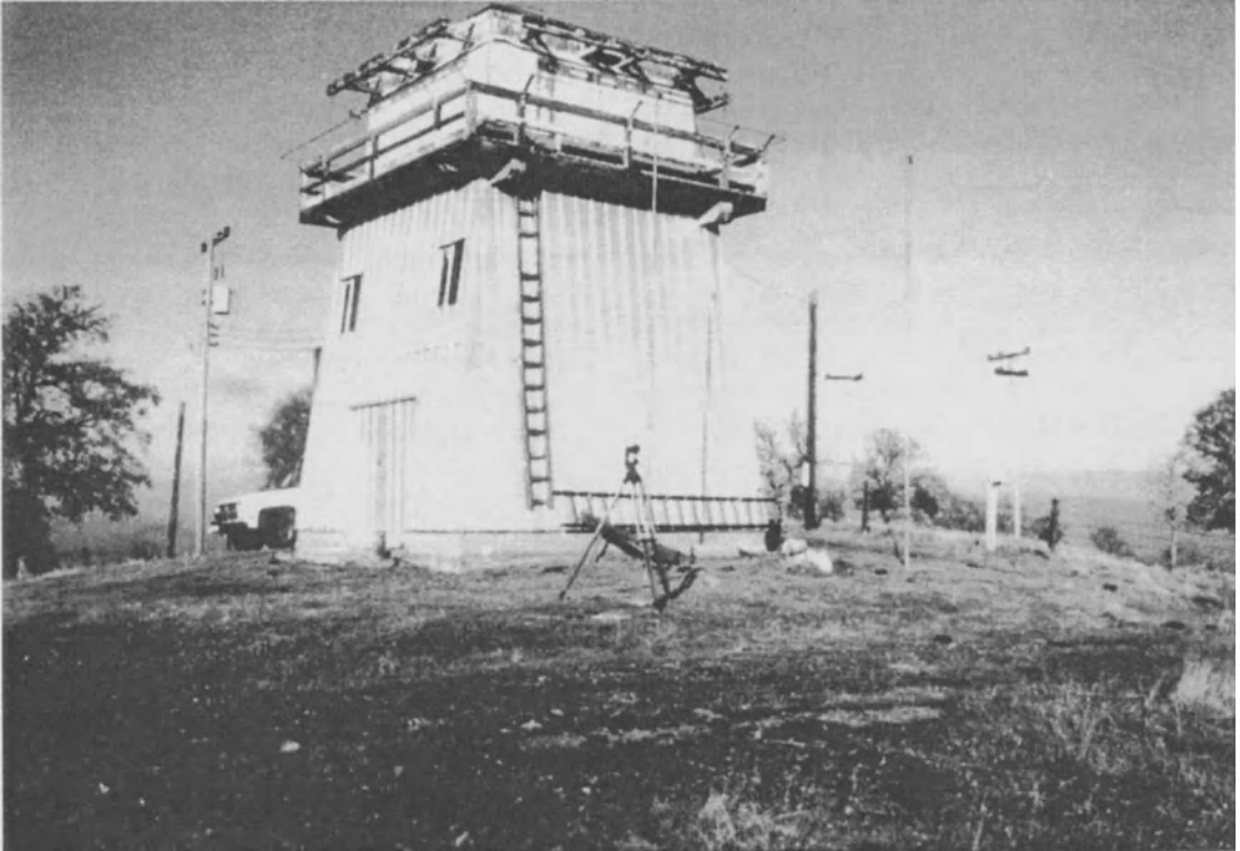
Figure 15-8. NGS station “Red top” showing a metal-sided building, the source of severe multipath conditions.
