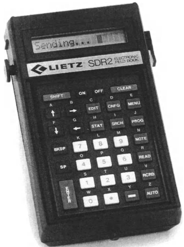
Figure 2-3. Lietz SDR2 electronic field book. (Courtesy of the Lietz Company.)
