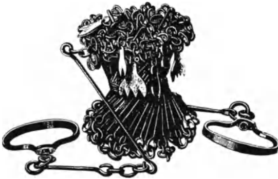
Figure 30-3. Surveyor's chain. (Courtesy of F. D. Uzes.)
