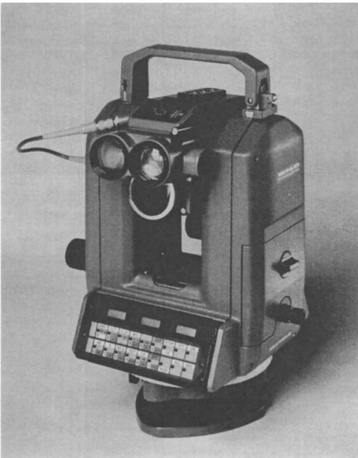
Figure 6-24. Wild T-2000 electric theodolite equipped with an EDM. (Courtesy of Wild Heerbrugg Instruments, Inc.)
