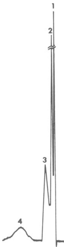
Figure 34. Separation of four chelating agents as Cu(II) complex: (1) \text{Cu}_2(\text{EGTA}) , (2) \text{Cu}(\text{NTA})^- , (3) \text{Cu}(\text{EDTA})^{2-} , (4) \text{Cu}(\text{CDTA})^{2-} . Column: Aminex A-14 anion exchange resin, 5 cm \times 2.1 mm (ID); detector: atomic absorption. (Reprinted from reference 121, courtesy of the American Chemical Society.)
