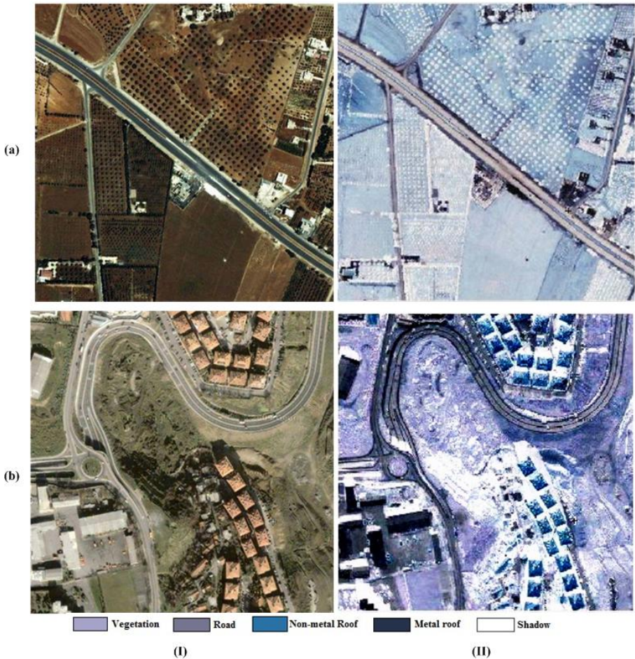
Fig. 2. ERICA based classified results of the emerging suburban area (a-b): (I) Input image; (II) Result of our proposed method
