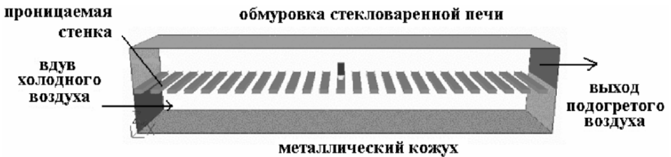
Figure 5. The third technique for cooling the external casing of a glass-melting furnace
