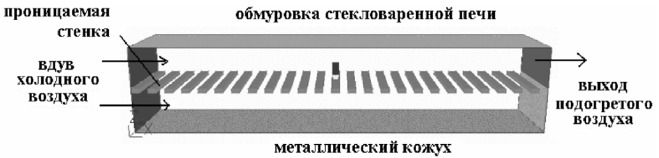
Figure 4. The second technique for cooling the external casing of a glass melting furnace
