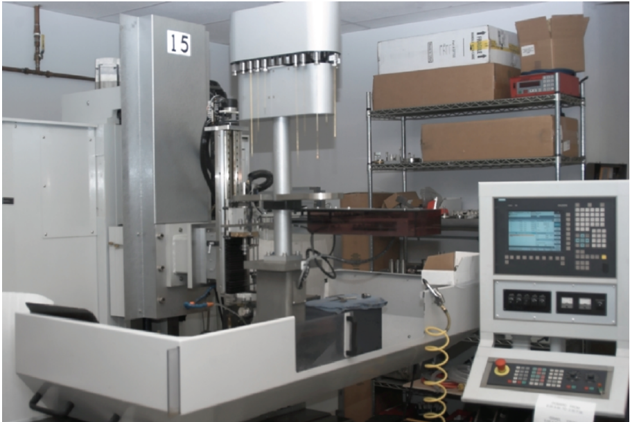
Figure 5. One of the EDM drilling machines installed at advanced EDM
