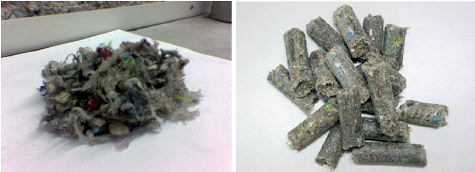
Figure 1. Manufactured fuels using MSW. (a) MSW fluff used to manufacture RDF from MBT plant; (b) pellets manufactured using extrusion
