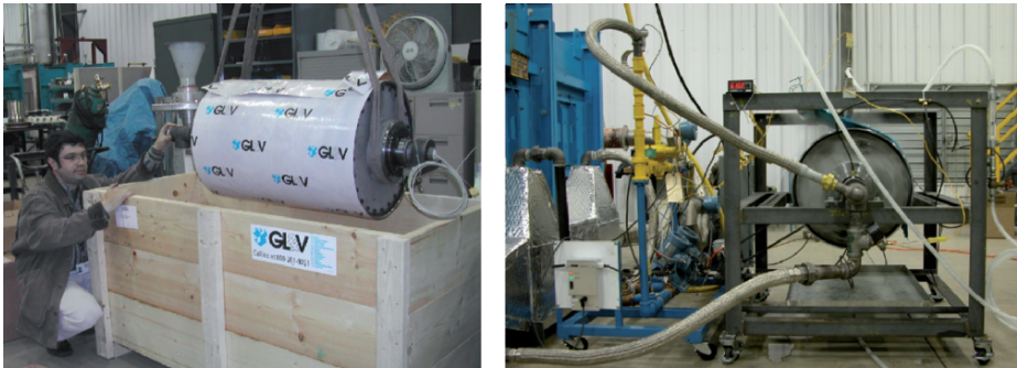
Figure 2. Pilot-scale GFPD and simulation rig equipped with the air/gas supply and heat recuperation
