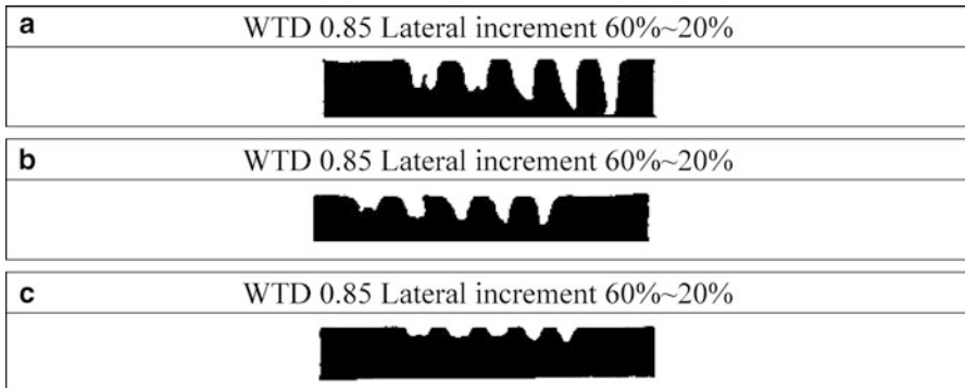
Fig. 6.25 The double-pass cut profile of various lateral feed increments [40], reprinted with permission. (a) WTD ratio less than 1.0. (b) WTD ratio between 1.0 and 2.0. (c) WTD ratio larger than 1.0
