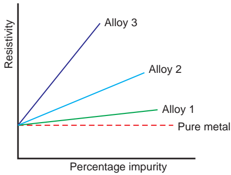
Figure 13.5 The variation of the resistivity of alloys with concentration of the alloying elements (schematic).
