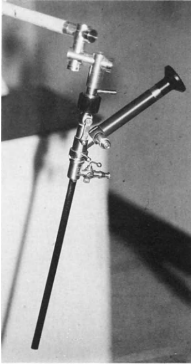
Fig. 5.1. Early prototype clinical laser urethrotome. based on the Storz nephroscope. ready for use.
