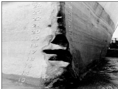
Figure 2 Close-up view of a vessel with damaged bow
