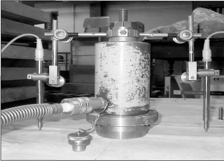
Figure 3 Testing apparatus complete with extractor and displacement transducers
