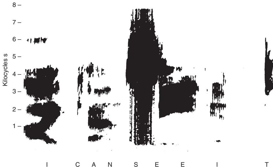
Figure 10.15 Sound spectrogram: 'I can see it'. The ordinate records the frequency of time in kHz and the abscissa records time. The sentence has been spoken very clearly. In the normal run of things the words are far less clearly separated. It is also found that the form of the consonants is strongly dependent on both the preceding and the following vowels. Note how the word 'it' is composed of two bursts of sound energy more widely separated than the bursts representing the different words.
