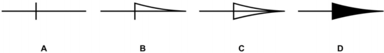
Figure 9. Method of drawing an arrowhead
