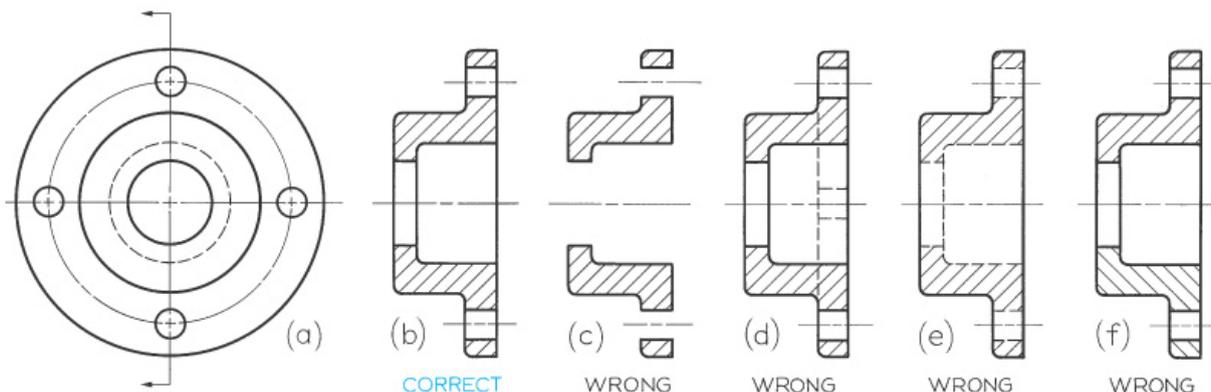
Figure: 1.10. (a) And (b) shows front view and section view
