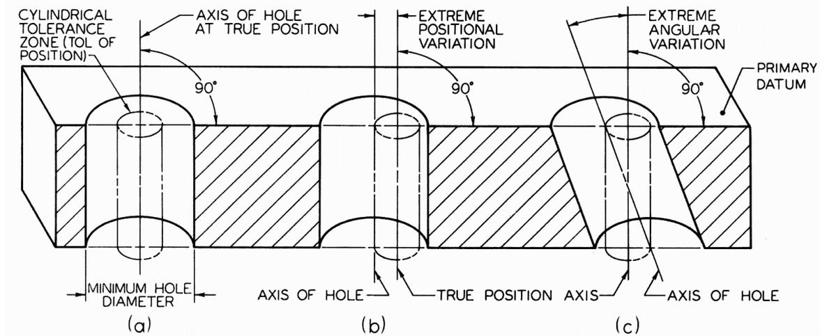
**Figure 6. Cylindrical Tolerance Zone**
