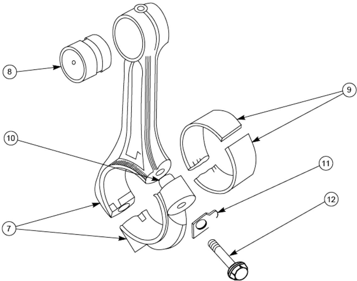
**Fig. 1.6** Exploded assembly drawing
