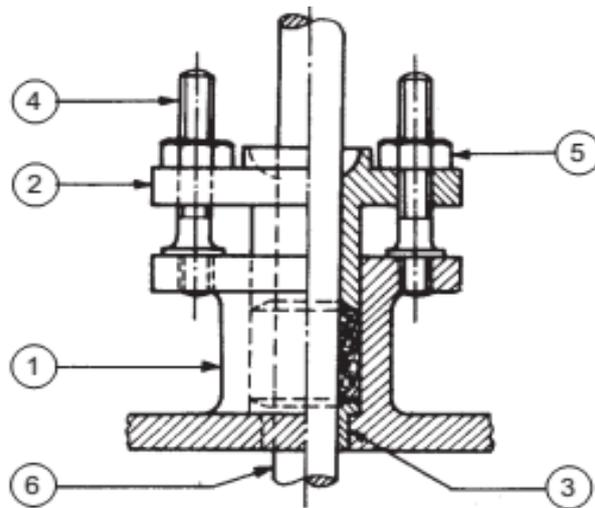
Figure 8. Stuffing Box Assembly
