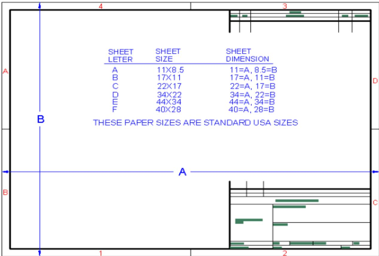
Figure 20 . Above is an example of a standard sheet with notation on its dimension
