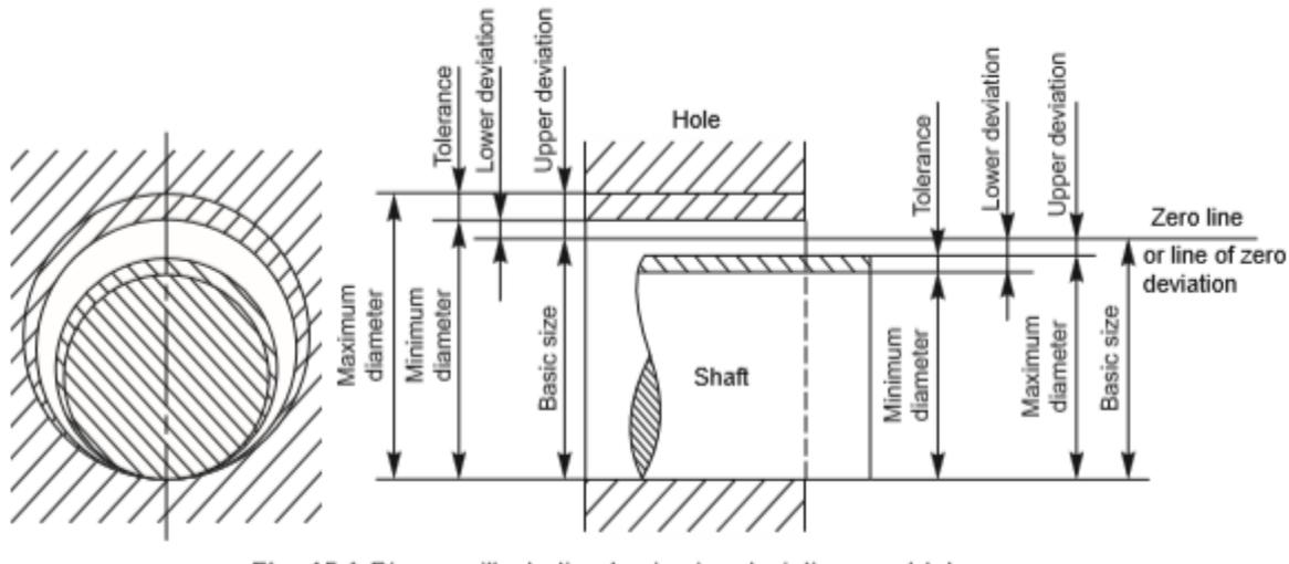
Figure 3. Diagram illustrating basic size deviations and tolerances
