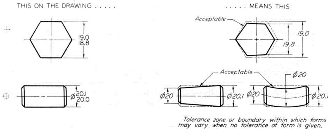
**Figure 19.** Acceptable Variations of Form – No Specified Tolerance of Form
