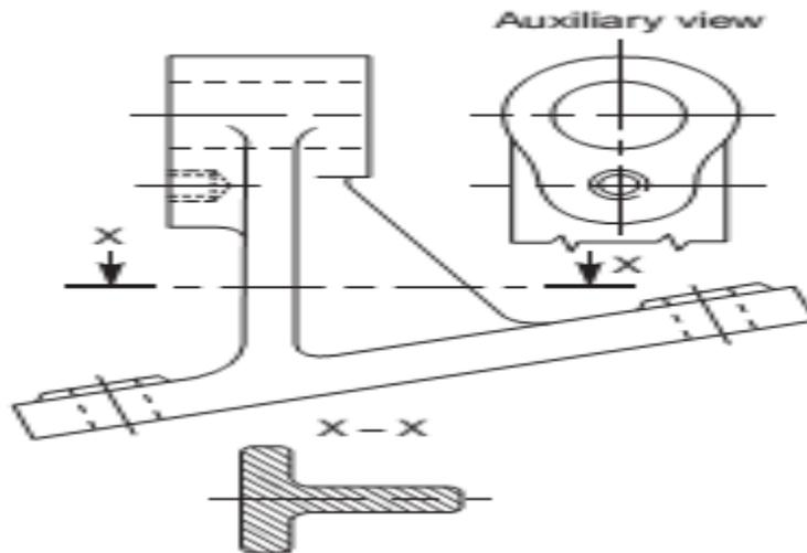
Figure 4. Auxiliary Section
