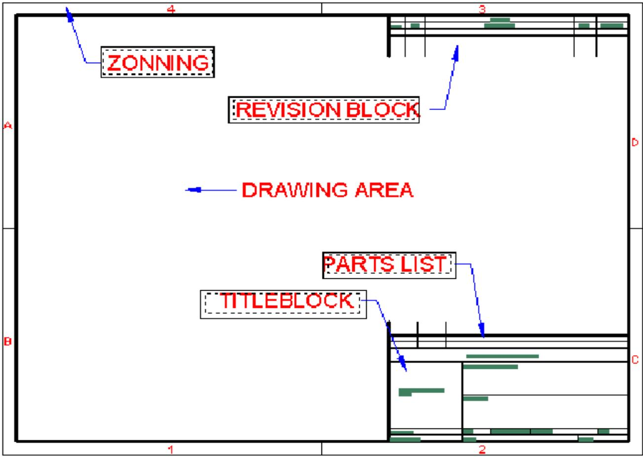
Figure19. Above is an example of a standard sheet with notation of its parts.
