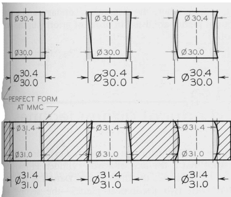
Figure 1. When only a tolerance of size is specified on a part, the limits prescribe the form of the part, as shown in these examples of shafts and holes with the same limits of tolerance.
