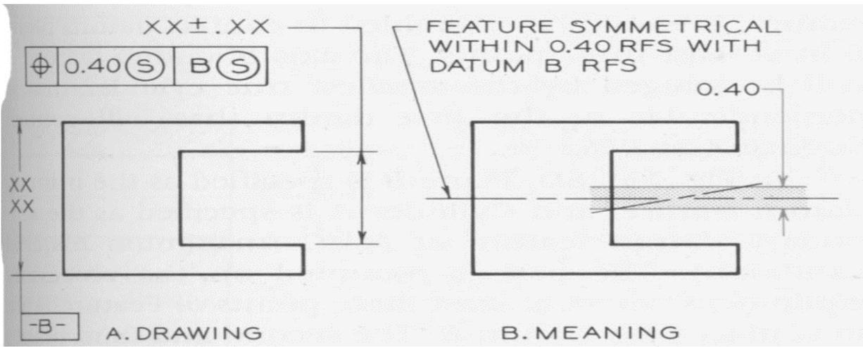
Figure 2. Tolerances of position should include a note of M, S, or L to indicate maximum material condition, regardless of feature size, or least material condition
