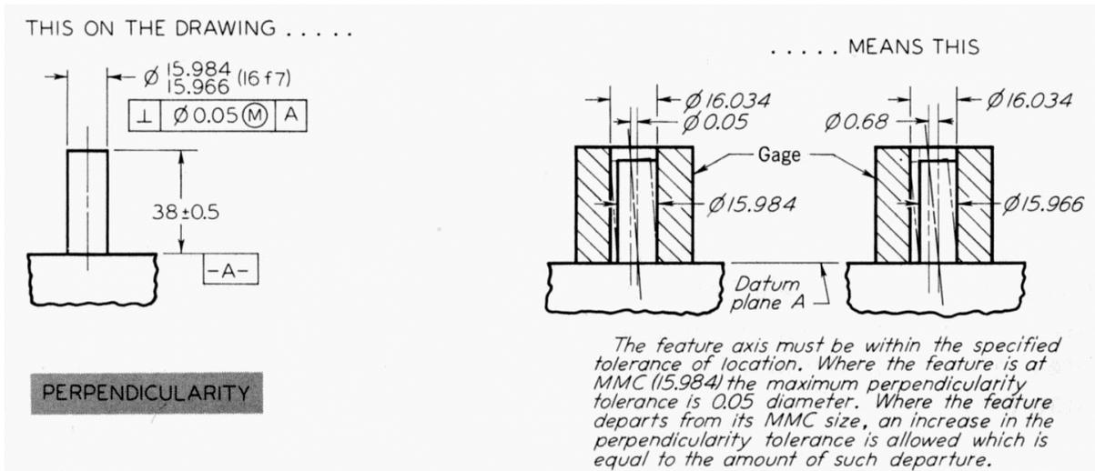
**Figure 26 . Specifying Perpendicularity for an Axis, Pin, or Boss**
