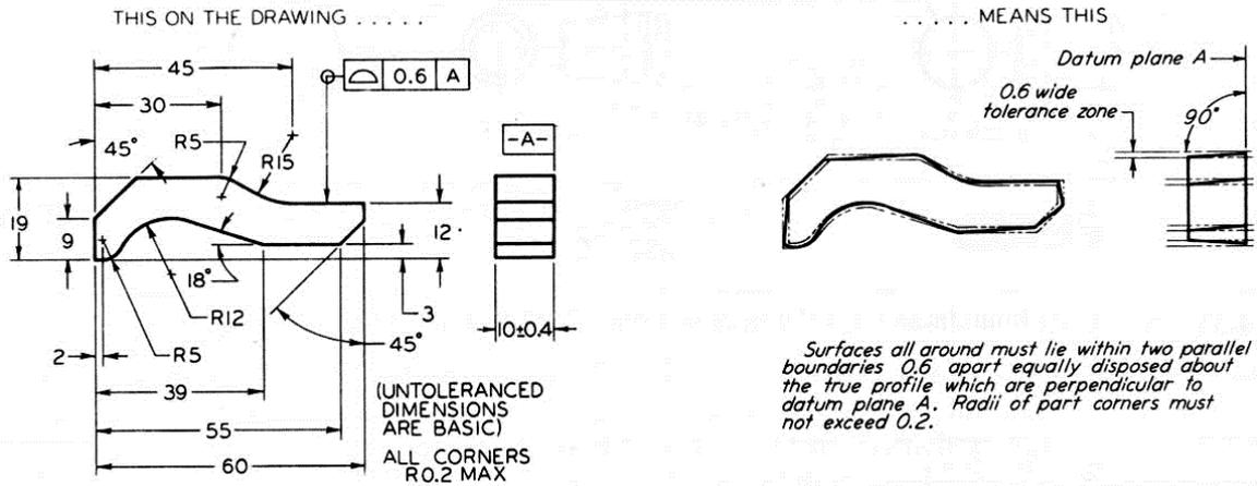
Figure 20. Specifying Profile of a Surface All Around
