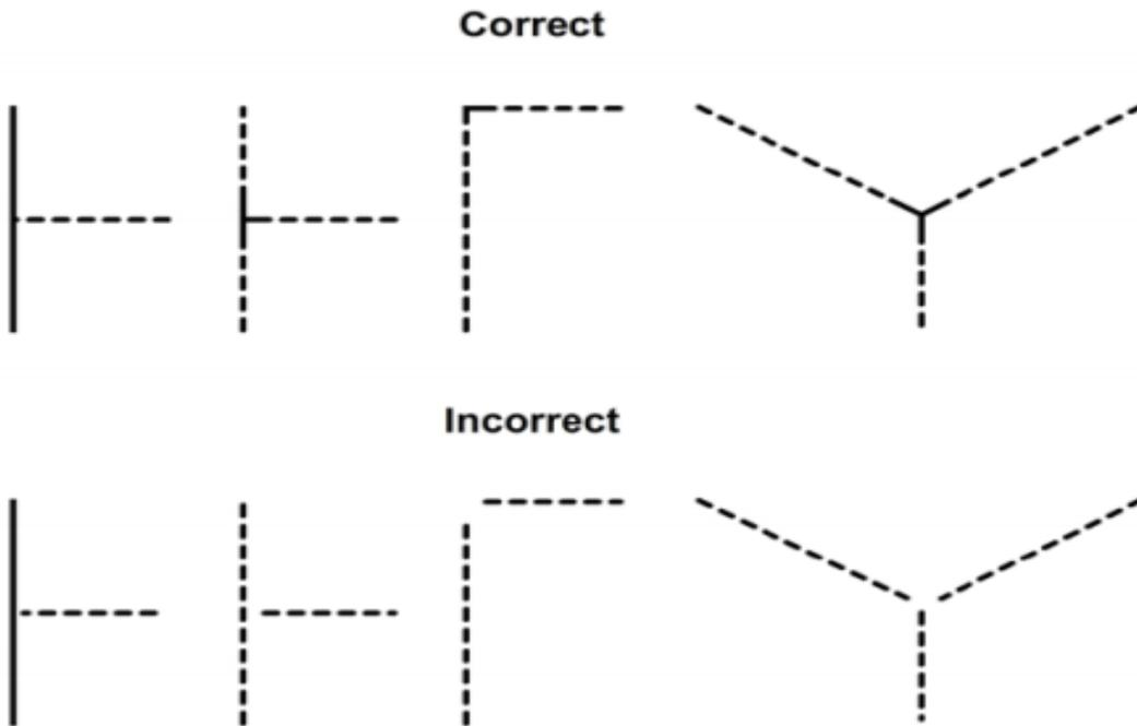
Figure 5 Correct and incorrect procedures for drawing adjoining lines.
