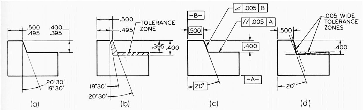
Figure11. Angular Tolerance Zones
