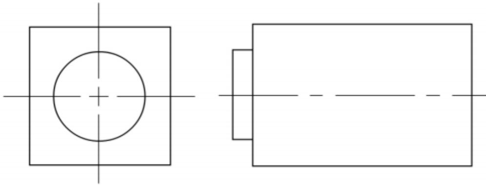
**Figure 3.** Use of visible edge line
