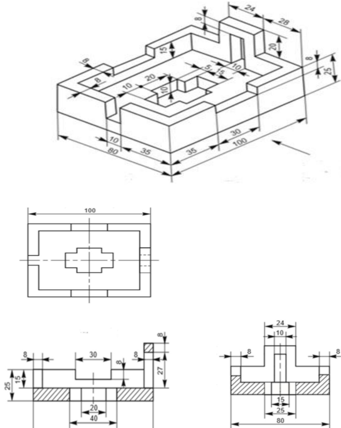
Figure 1 Machine Block
