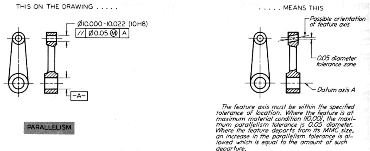
**Figure 24.** Specifying Parallelism for an Axis Feature at MMC
