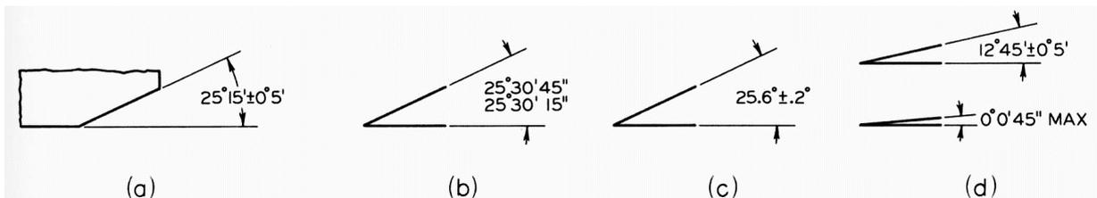
Figure10. Tolerances of Angles
