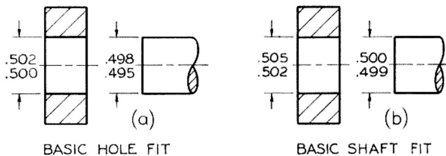
**Figure 11.** Basic Hole and Basic Shaft Systems
