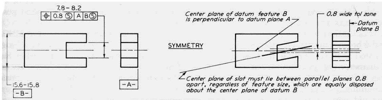
Figure 9. Positional Tolerance for Symmetry
