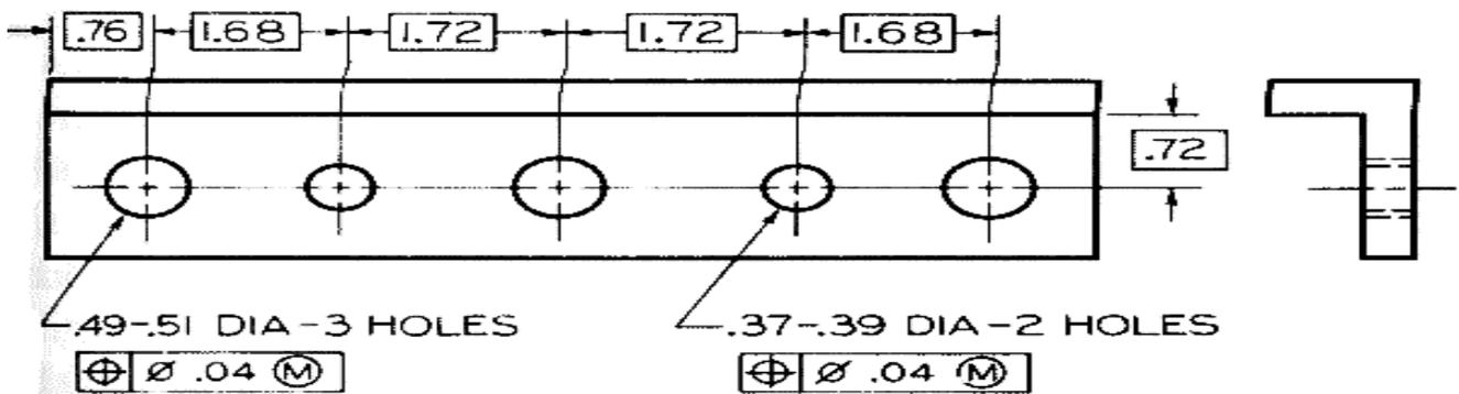
**Figure 8.** No Tolerance Accumulation
