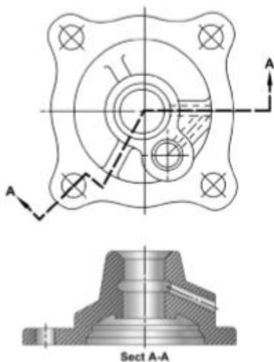
**Figure 13. Use of an offset section**
