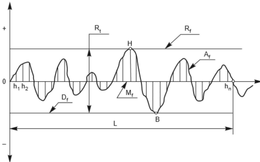
Figure 27 Surface roughness
