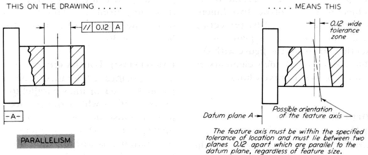
**Figure 23.** Specifying Parallelism for an Axis Feature RFS
