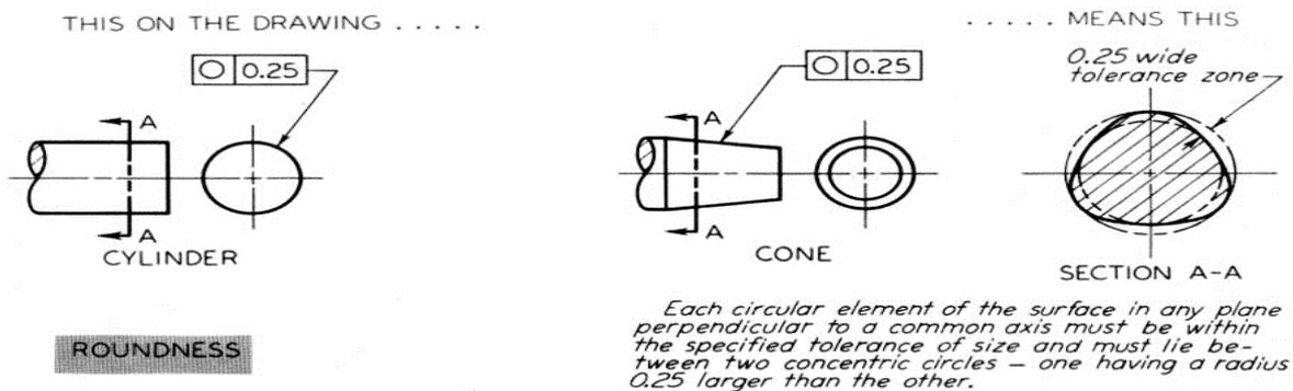
Figure 17. Specifying Roundness for a Cylinder or Cone
