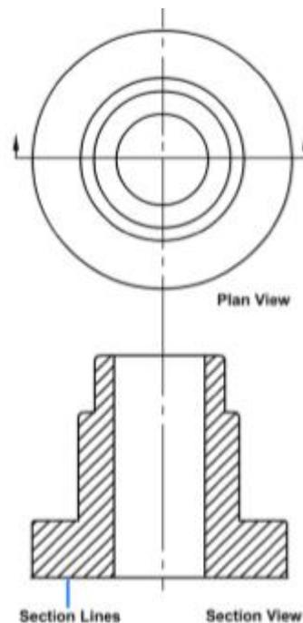
**Figure 14.** Drawing of a plan view and a full section
