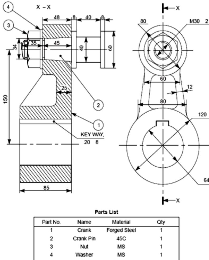
Figure 1.3. Assembly Drawing
