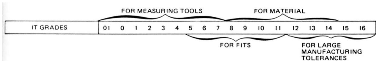
Figure 2. Practical Use of International Tolerance Grades
