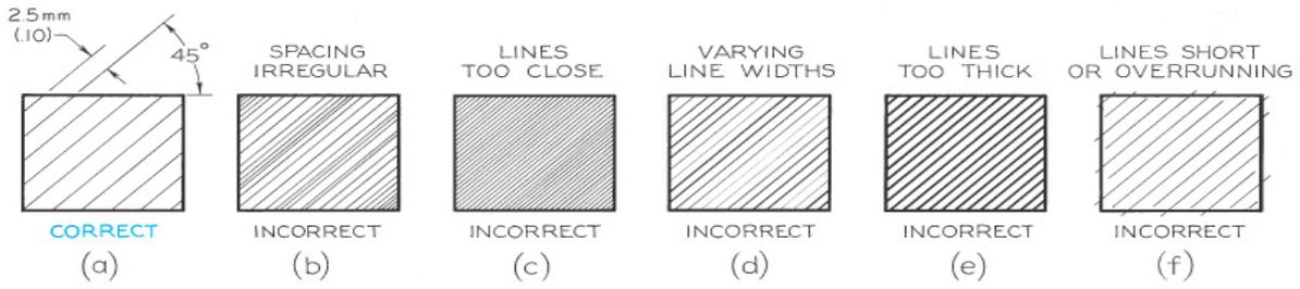
Figure1. 11. Shading with thin solid lines (Hatching)
