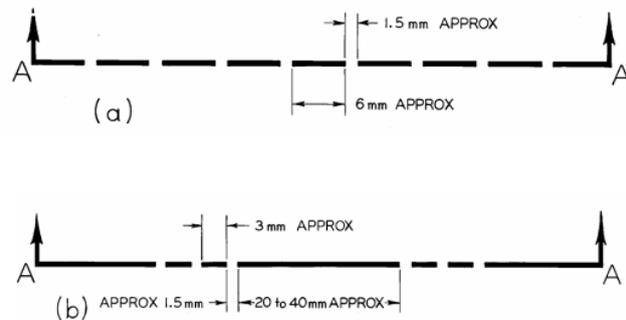
Figure 1.13: Cutting Plane Line
