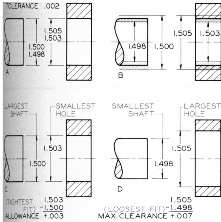
**Figure 6.** The allowance (tightest fit) between these assembled parts is +0.003". The maximum clearance is 0.007".
