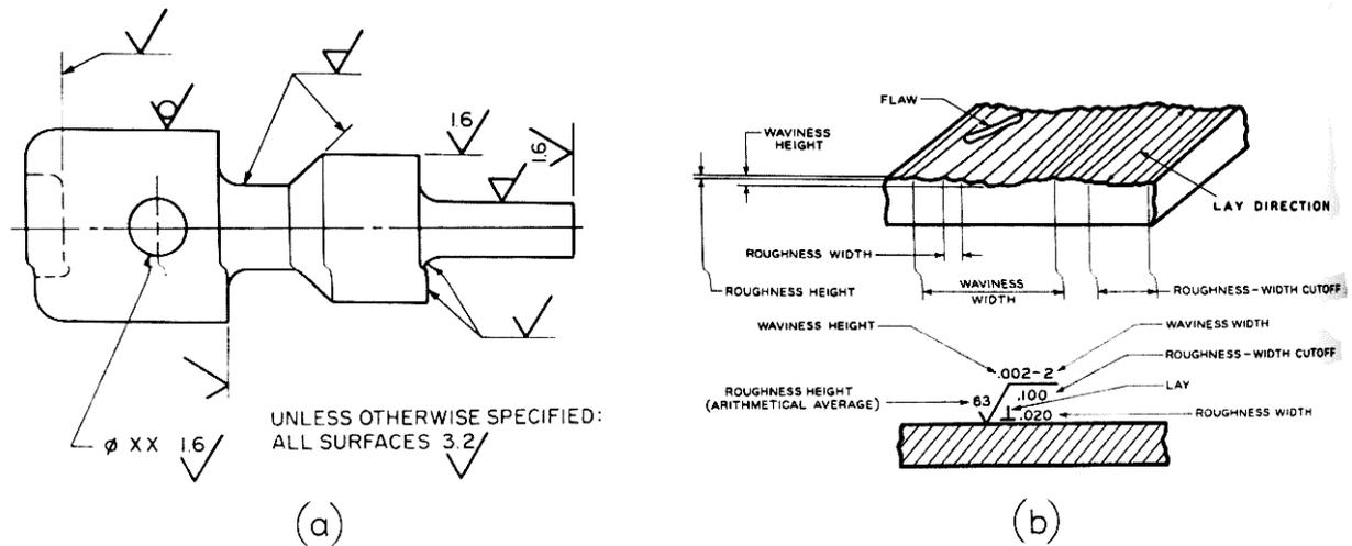
**Figure 3.** Application of Surface Texture Symbols and Surface Characteristics
