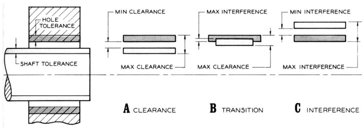
Figure 14. Types of fit (A) A clearance fit; (B) a transition fit where there can be interference or a clearance; and (C) an interference fit, where the parts must be forced together.
