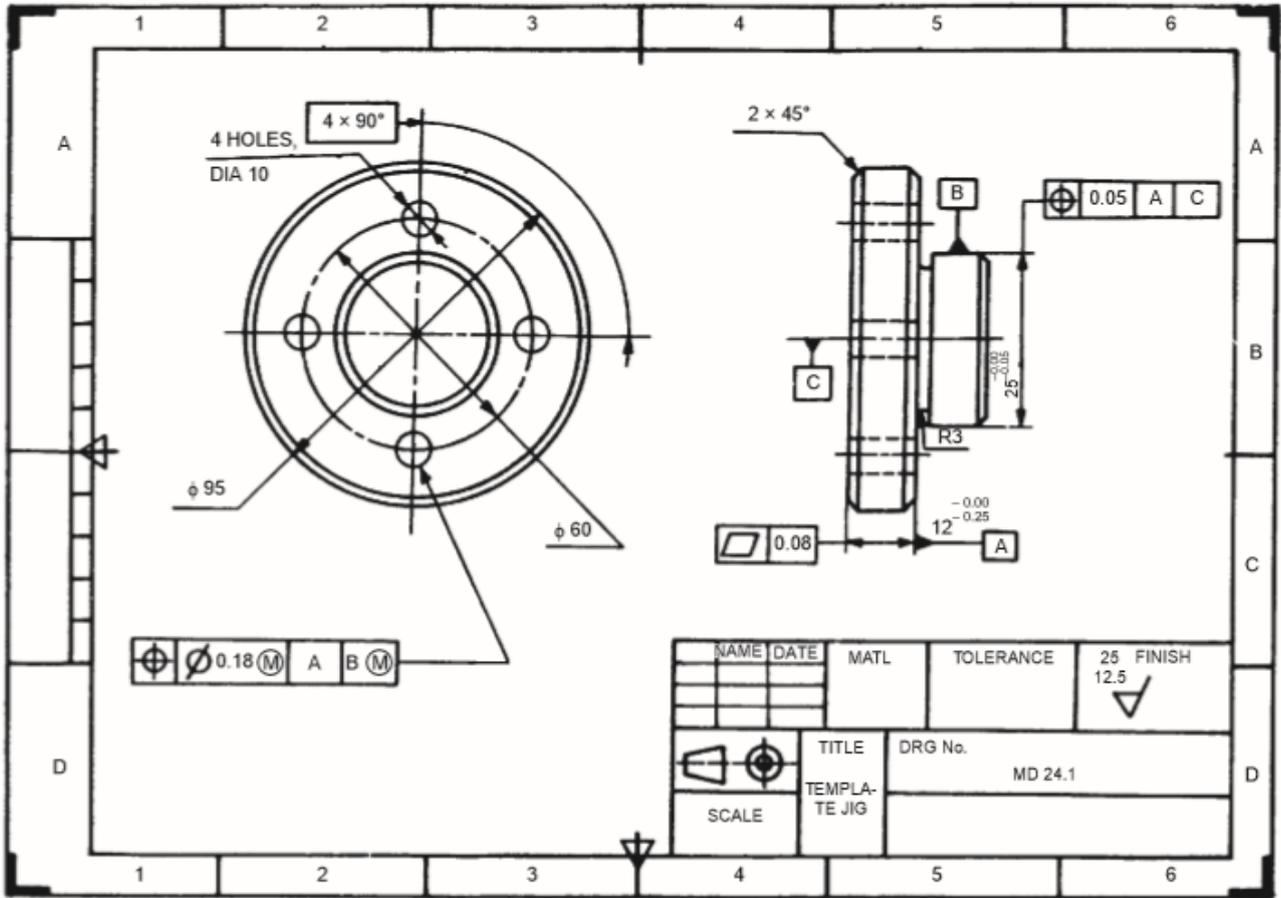
Figure 1.1: Detail drawing of template jig
