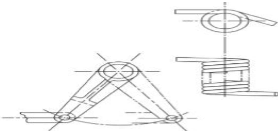
**Figure 11 — Use of phantom lines.**
