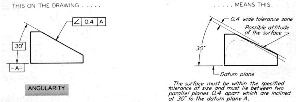
Figure 21. Specifying Angularity for a Plane Surface
