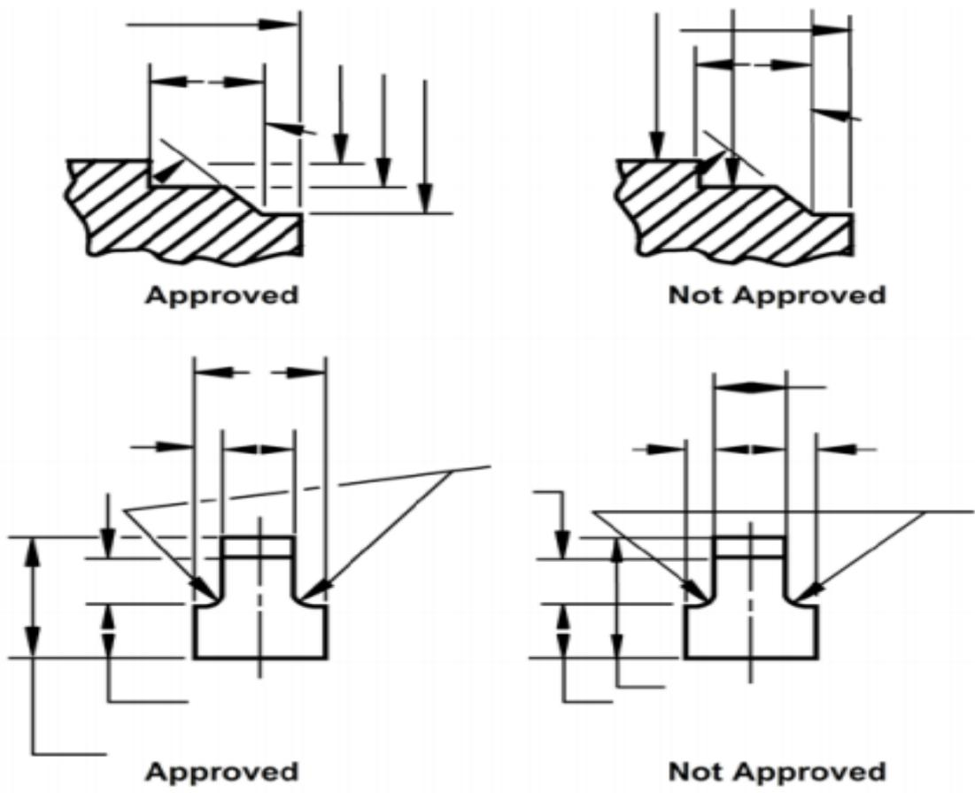
Figure 8. Breaking extension lines and leaders at points of intersections.
