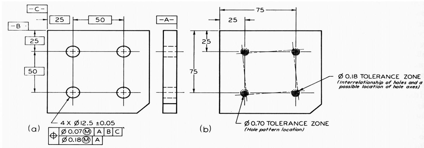
**Figure 5. True-Position Dimensioning**
