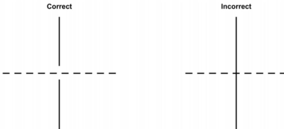
Figure 6 Correct and incorrect procedures for drawing a hidden edge line that intersects a visible edge line.
