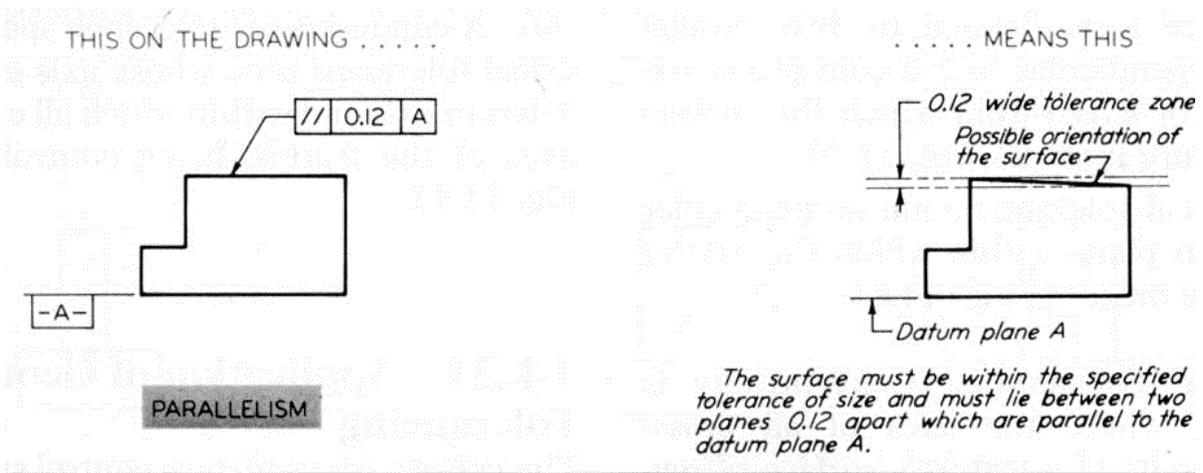
**Figure 22.** Specifying Parallelism for a Plane Surface
