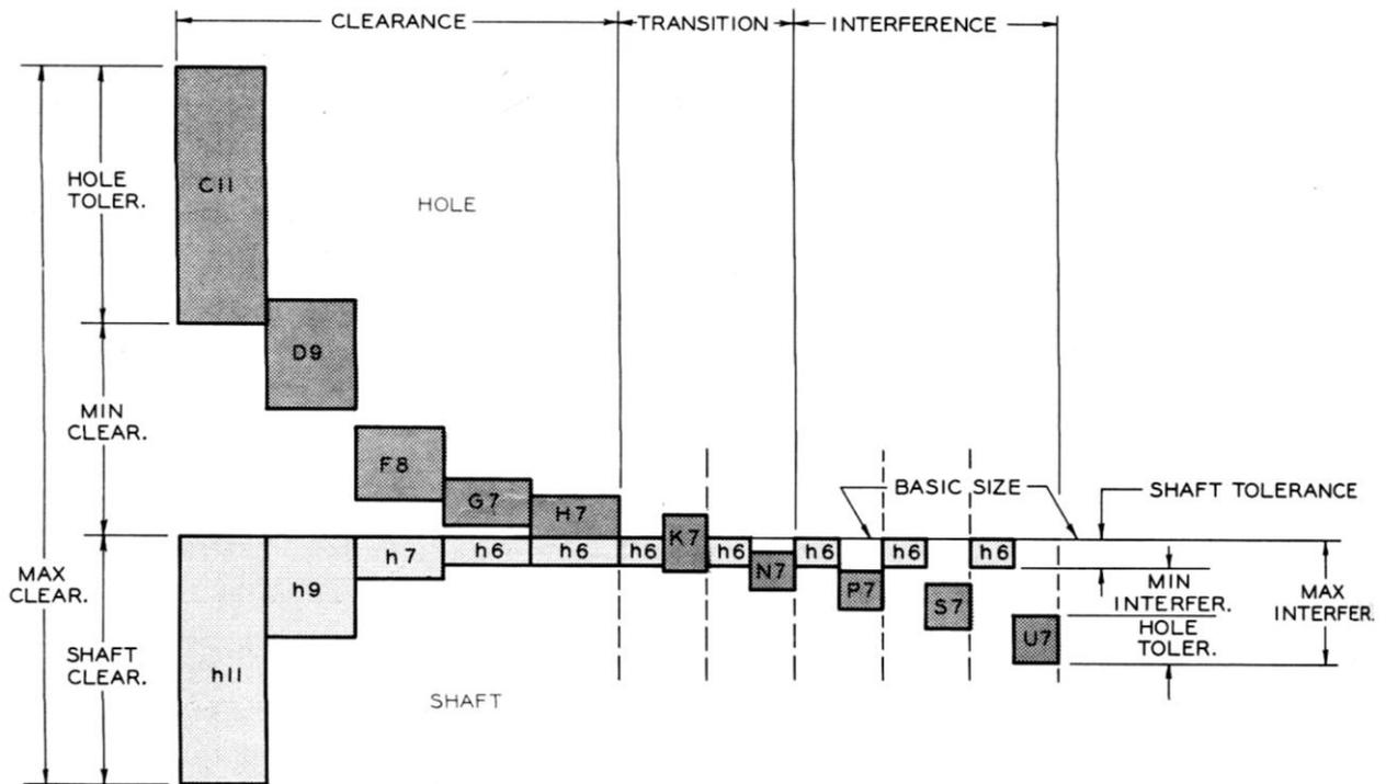
Figure 15. The preferred fits for a shaft basis system. These fits correspond to those given in Table 2.
